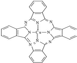
Figure 7.11 Structure of Copper Phthalocyanine Blue
