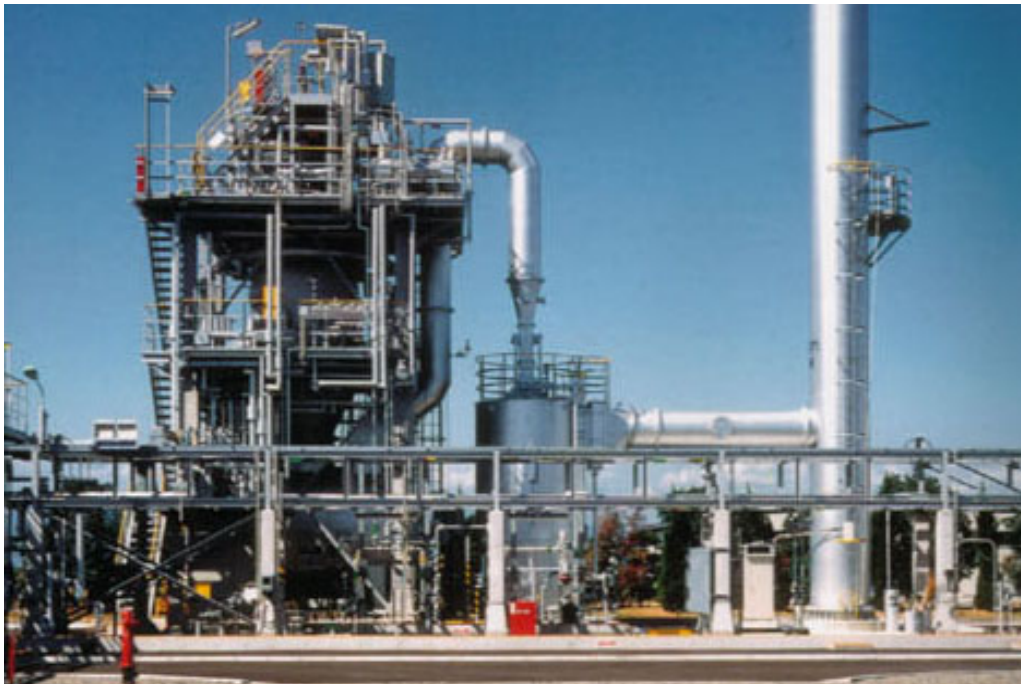
Figure 3.8. Scheme of waste liquid treatment unit. Nittetu Chemical Engineering Co., Tokyo 174-0041 Japan
