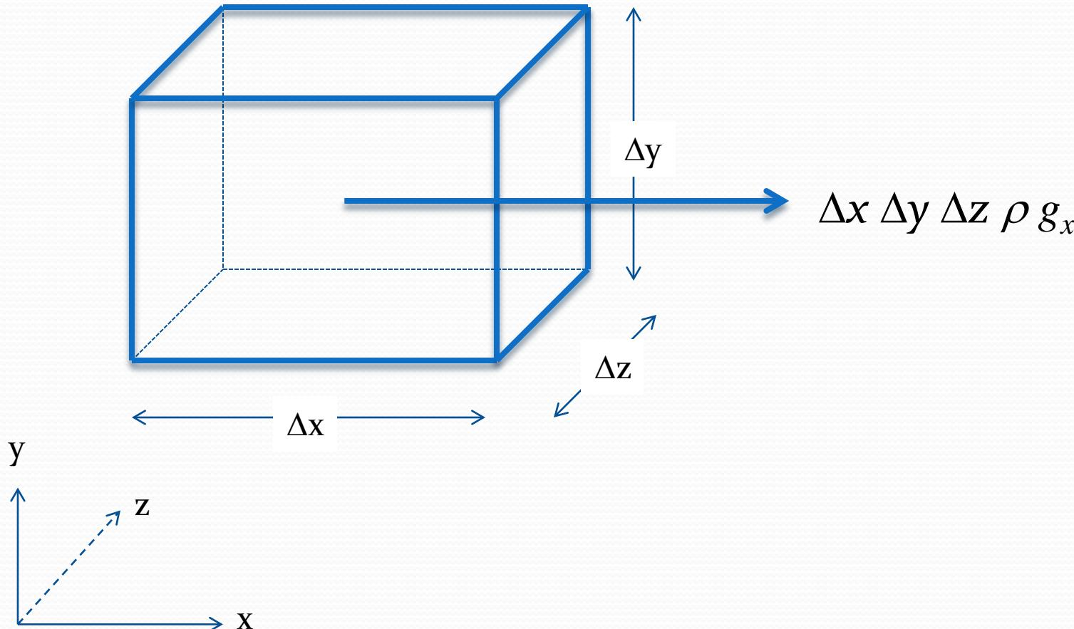
$$\left[ \rho v_x v_x \Big|_x - \rho v_x v_x \Big|_{x+\Delta x} \right] \Delta y \Delta z + \left[ \rho v_y v_x \Big|_y - \rho v_y v_x \Big|_{y+\Delta y} \right] \Delta x \Delta z + \left[ \rho v_z v_x \Big|_z - \rho v_z v_x \Big|_{z+\Delta z} \right] \Delta x \Delta y +$$
