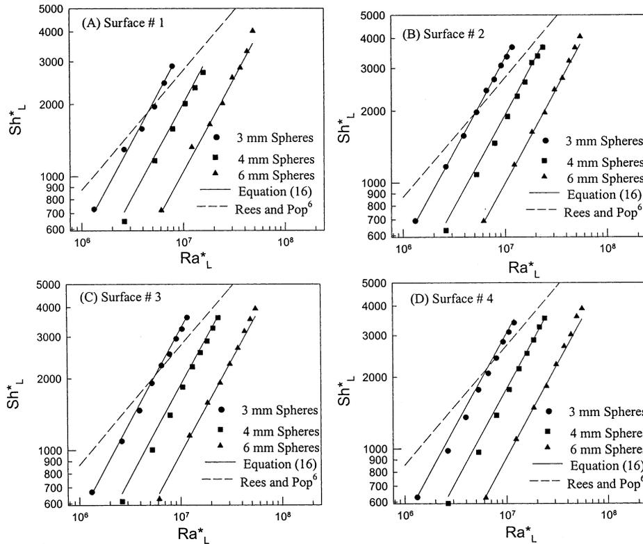
**Figure 7.** Experimental and predicted values of  $Sh_L^*$ .
