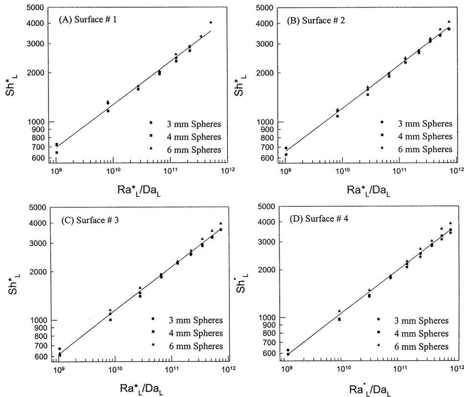
**Figure 5.** Variation of average modified Sherwood number ( $Sh_L^*$ ) with  $Ra_L^*/Da_L$  for (A) surface 1, (B) surface 2, (C) surface 3, and (D) surface 4.
