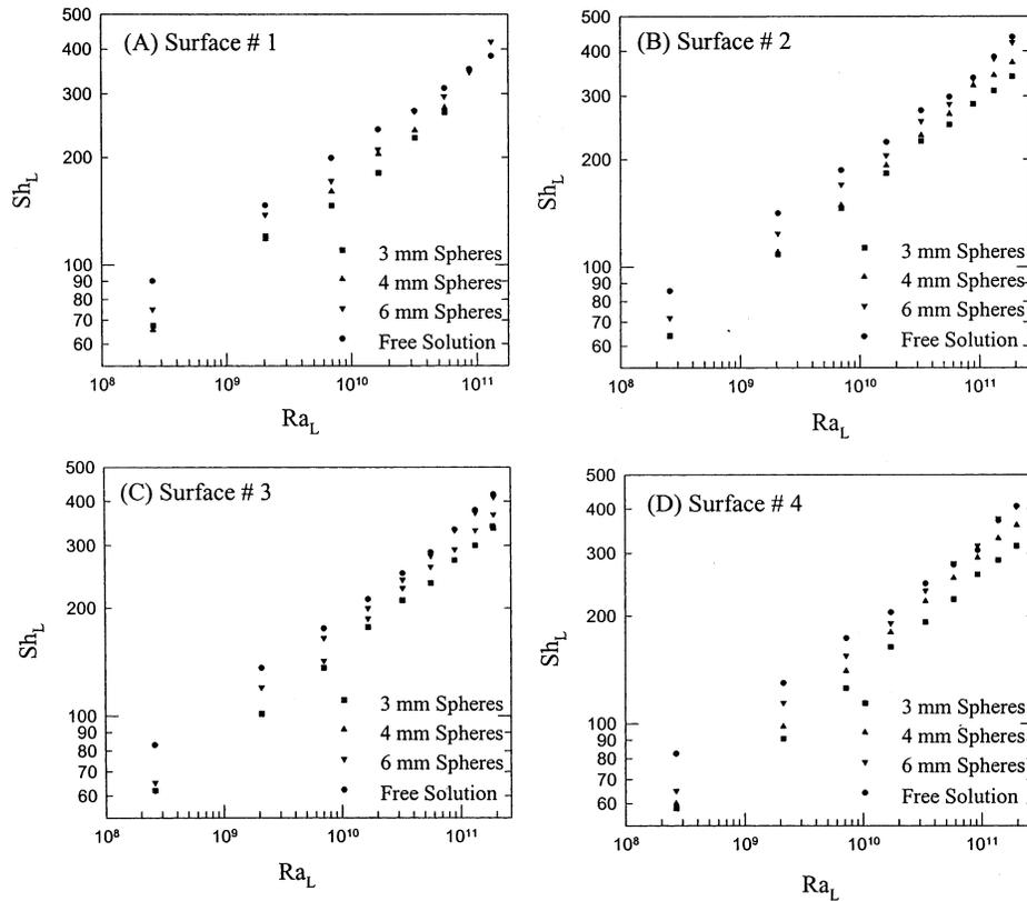
**Figure 4.** Variation of average Sherwood number with Rayleigh number in various porous media for (A) surface 1, (B) surface 2, (C) surface 3, and (D) surface 4.
