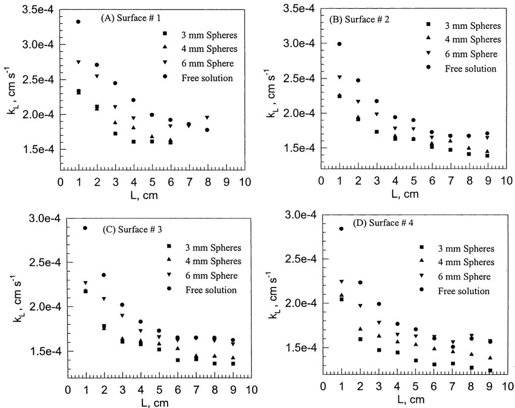
**Figure 3.** Variation of average mass transfer with vertical distance in various porous media for (A) surface 1, (B) surface 2, (C) surface 3, and (D) surface 4.
