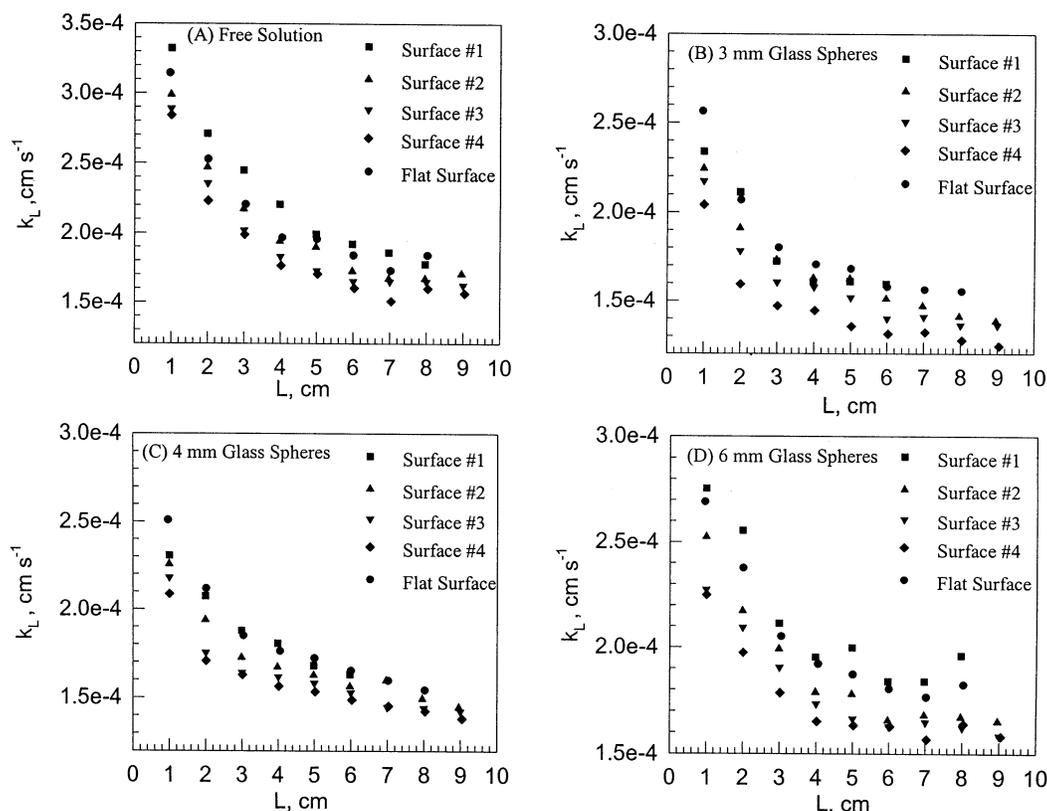
**Figure 1.** Variation of average mass transfer with vertical distance of various wavy surfaces in (A) free solution, (B) saturated packing of 3-mm glass spheres, (C) saturated packing of 4-mm glass spheres, and (D) saturated packing of 6-mm glass spheres.
