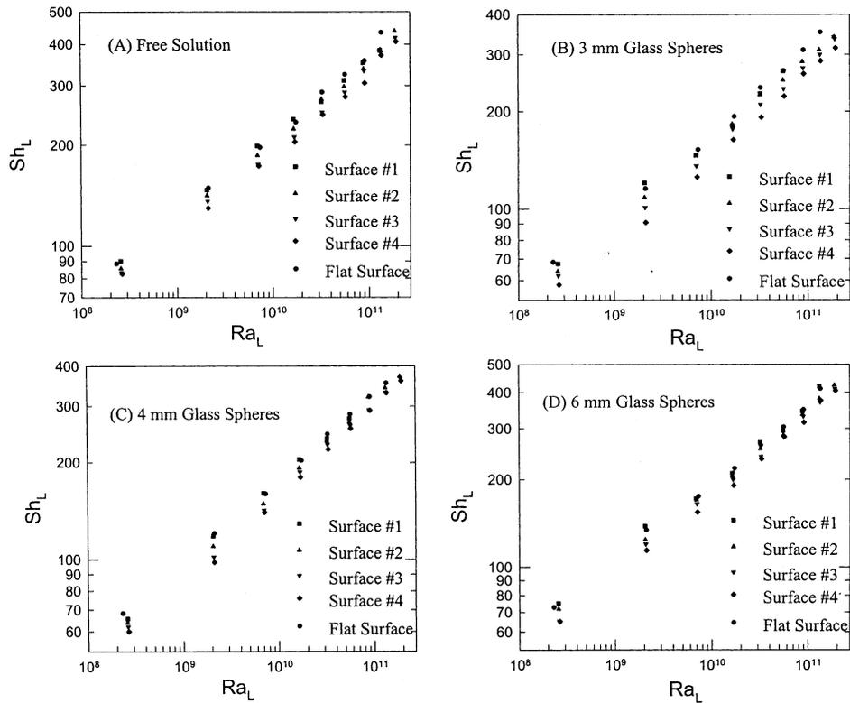
**Figure 2.** Variation of average Sherwood number with Rayleigh number of various wavy surfaces in (A) free solution, (B) saturated packing of 3-mm glass spheres, (C) saturated packing of 4-mm glass spheres, and (D) saturated packing of 6-mm glass spheres.
