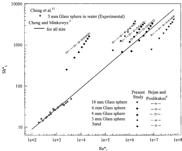
**Figure 5.** Comparison of experimental mass-transfer data with models due to Cheng and Minkowycz<sup>3</sup> and Bejan and Poulikakos<sup>6</sup> and experiments of Cheng et al.<sup>11</sup>
