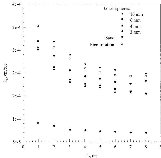
**Figure 3.** Average mass-transfer coefficients for vertical surfaces embedded in different packing materials.
