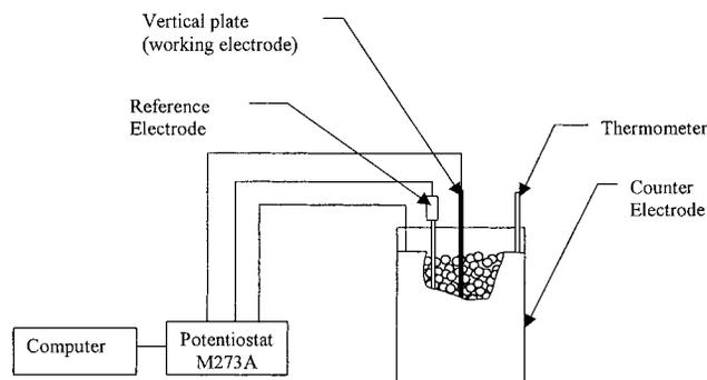
Figure 1. Experimental setup for measuring the limiting current.
