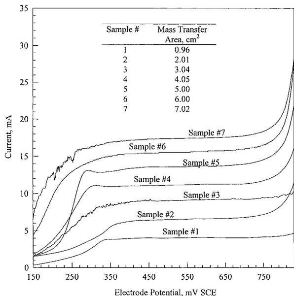
**Figure 2.** Potentiostatic polarization curves showing limiting currents for vertical copper plates in a  $\text{CuSO}_4$  solution.
