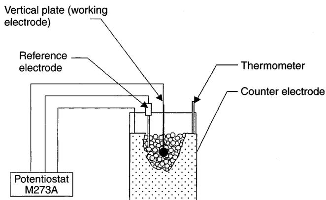
Fig. 1. Experimental set-up for measuring limiting current
