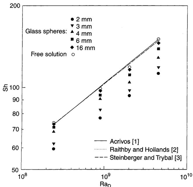
Fig. 5. Average Sherwood number versus Rayleigh number plots for different packing particles
