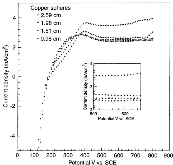
Fig. 2. Potentiostatic polarization curves of copper spheres in free solution
