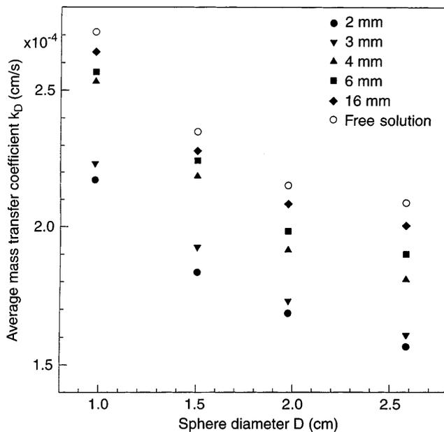
Fig. 4. Average mass transfer coefficient versus diameter of sphere for different packing particles
