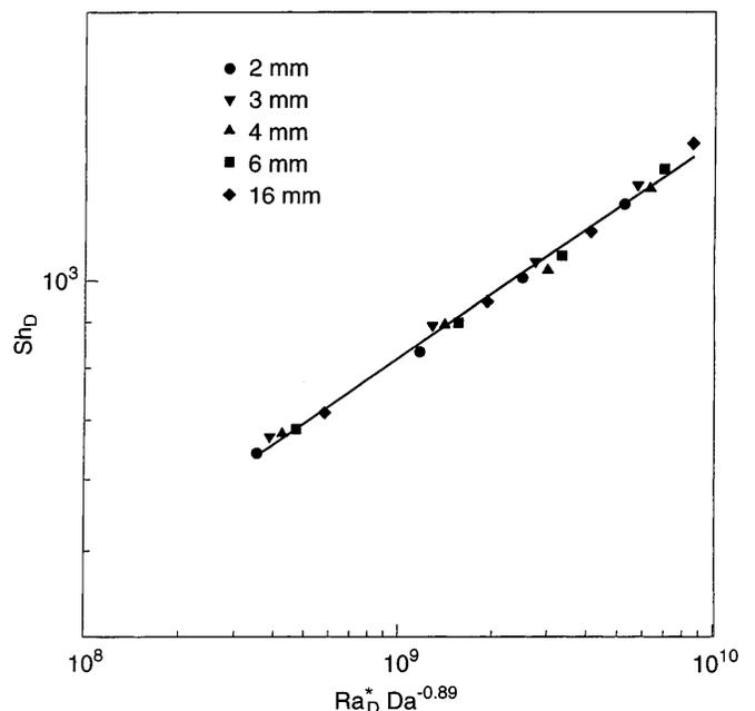
Fig. 7. Average Sherwood number versus  $Ra_D^* Da^{-0.89}$  curves for spherical particles
