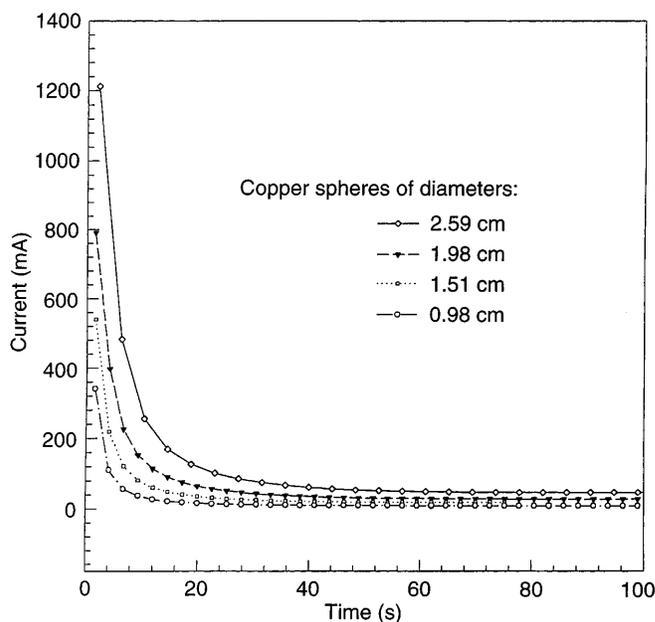
Fig. 3. Chronoamperometric curves of different copper spheres suspended in free solution at 550 mV SCE
