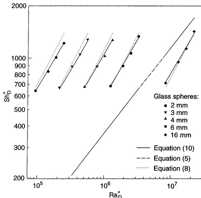
Fig. 6. Variation of Sherwood number with modified Rayleigh number for different packing particles
