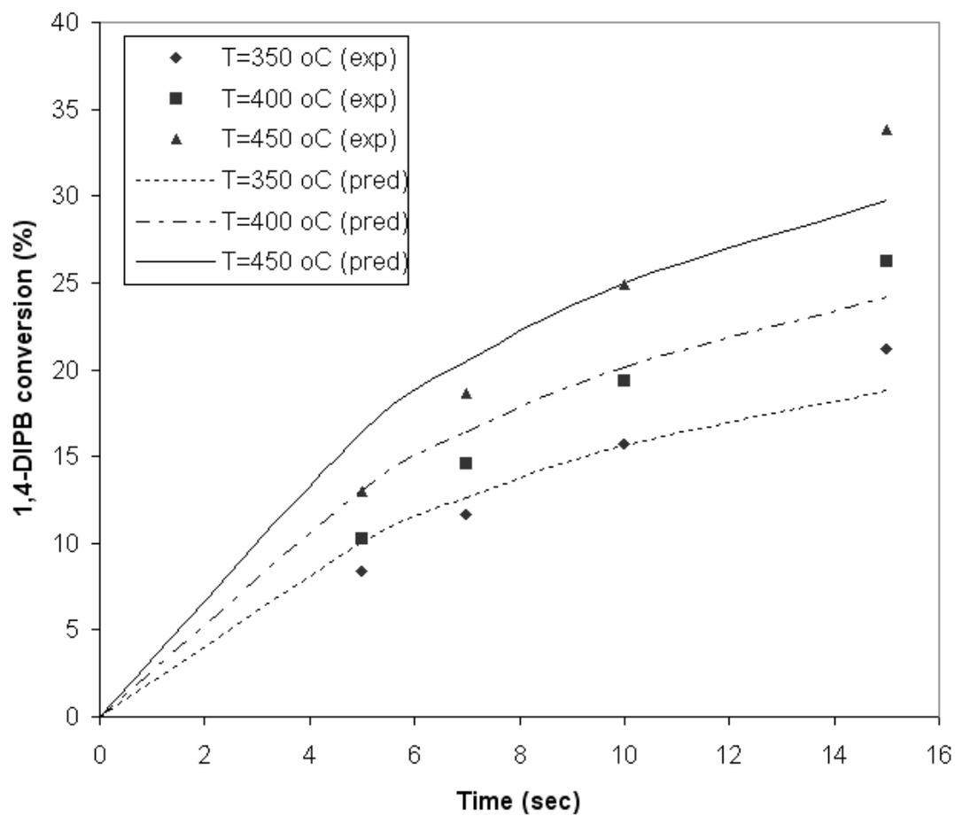
Figure 9: Modeling 1,4-DIPB conversion (FCC-B). Decay function based on time on stream (TOS)
