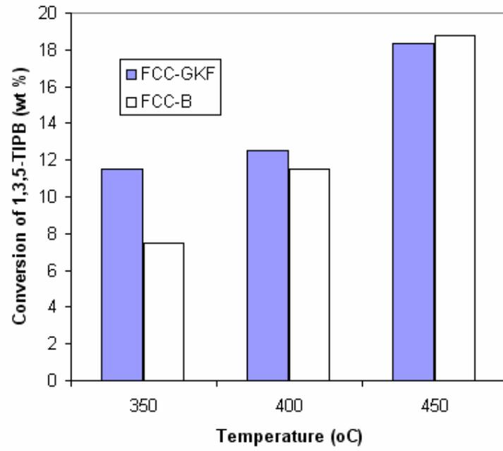
Figure 5: 1,3,5-TIPB conversion at 7-s reaction time and various temperatures
