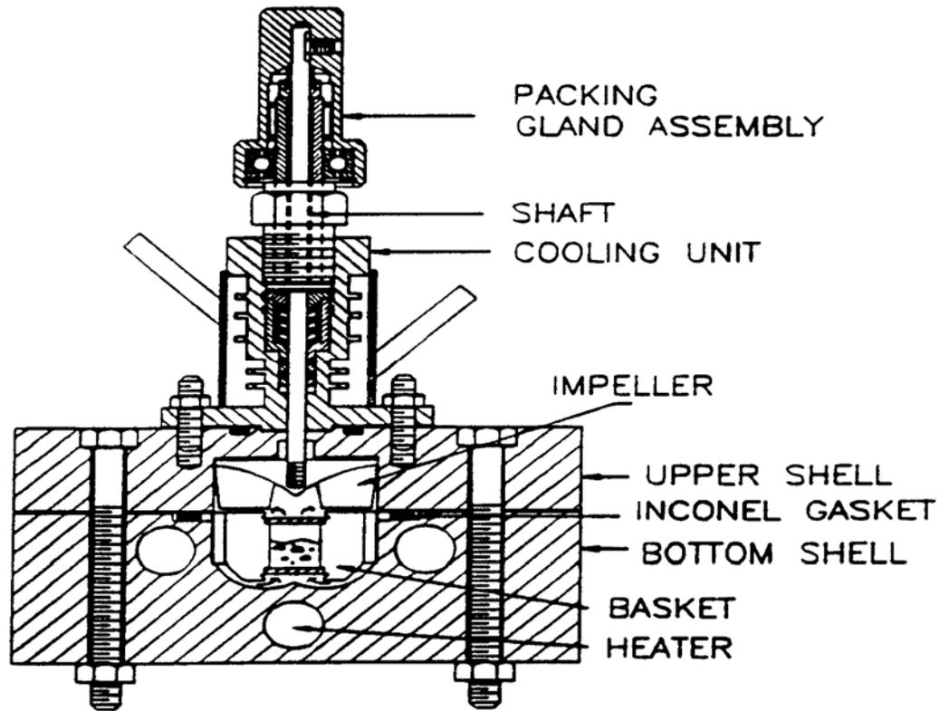
Figure 1: Schematic Diagram of the Riser Simulator
