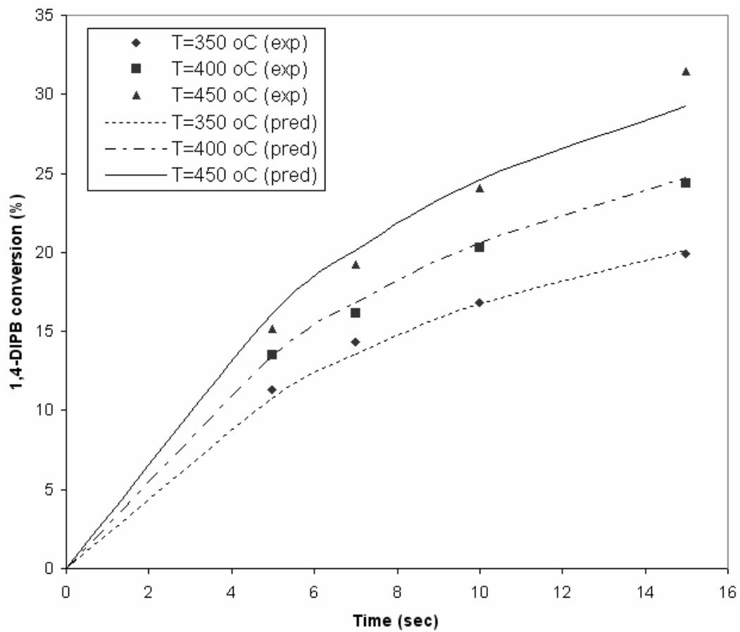
Figure 8: Modeling 1,4-DIPB conversion (FCC-GKF). Decay function based on time on stream (TOS)
