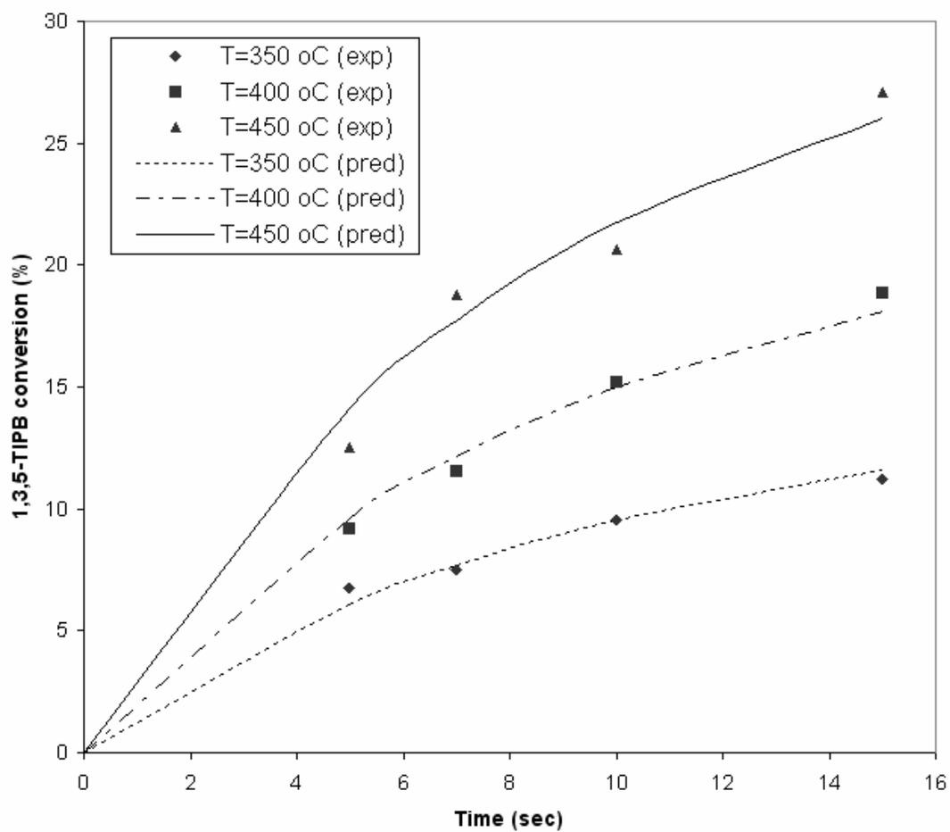
Figure 4: Modeling 1,3,5-TIPB conversion (FCC-B). Decay function based on time on stream (TOS)
