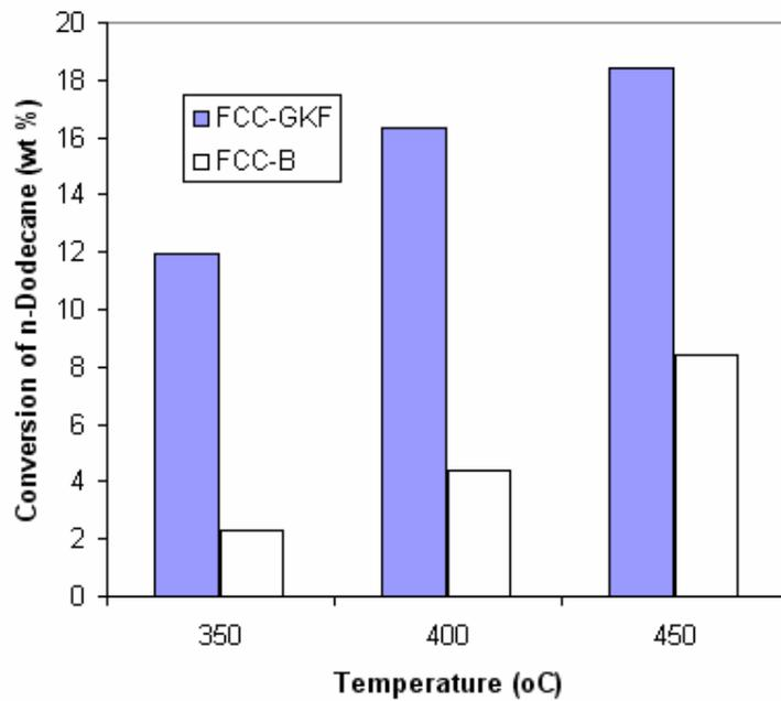
Figure 14: Dodecane conversion at 7-s reaction time and various temperatures
