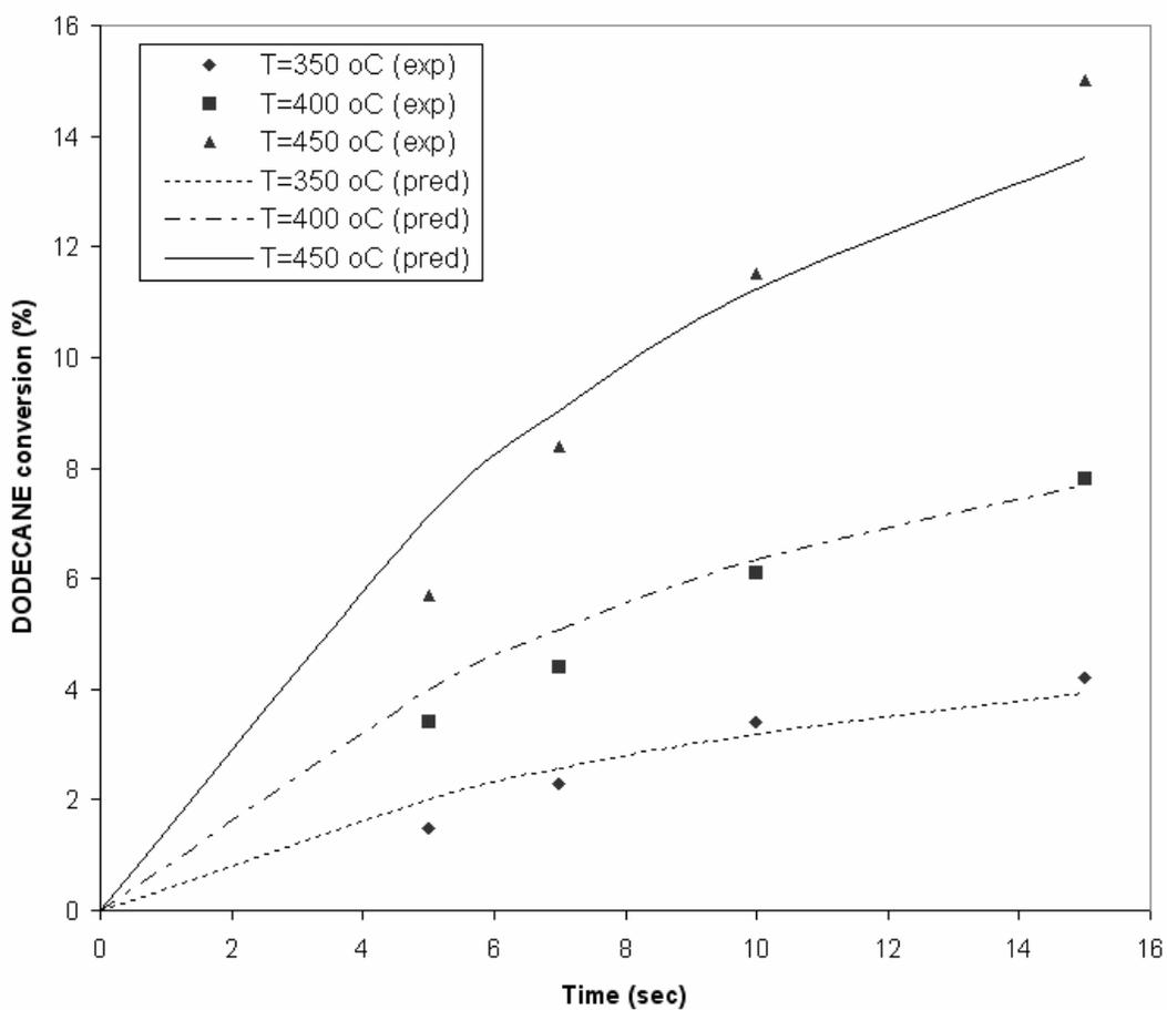
Figure 13: Modeling DODECANE conversion (FCC-B). Decay function based on time on stream (TOS)
