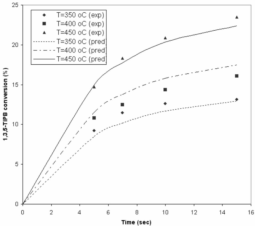
Figure 3: Modeling 1,3,5-TIPB conversion (FCC-GKF). Decay function based on time on stream (TOS)
