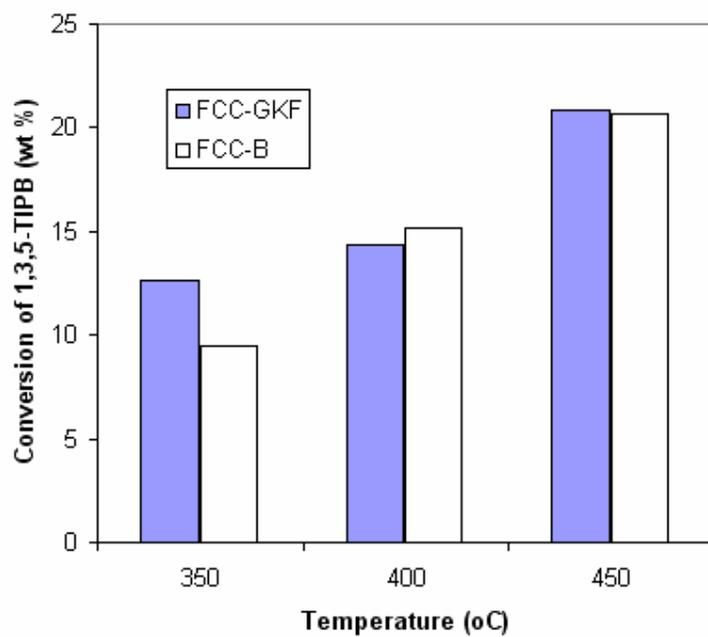
Figure 6: 1,3,5-TIPB conversion at 10-s reaction time and various temperatures
