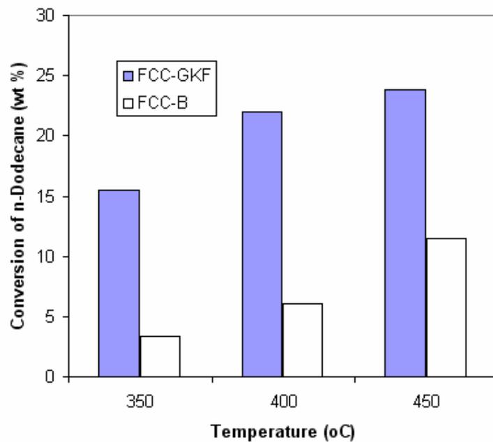
Figure 15: Dodecane conversion at 10-s reaction time and various temperatures
