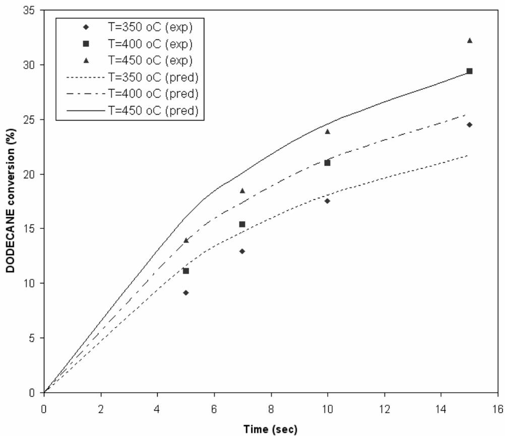
Figure 12: Modeling DODECANE conversion (FCC-GKF). Decay function based on time on stream (TOS)
