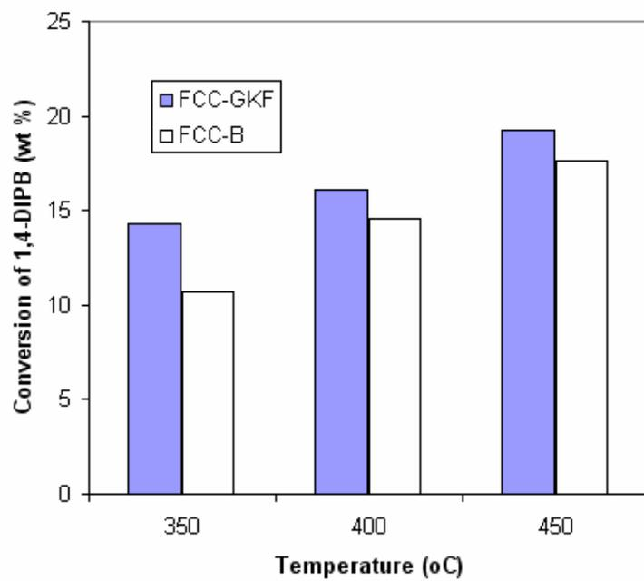
Figure 10: 1,4-DIPB conversion at 7-s reaction time and various temperatures
