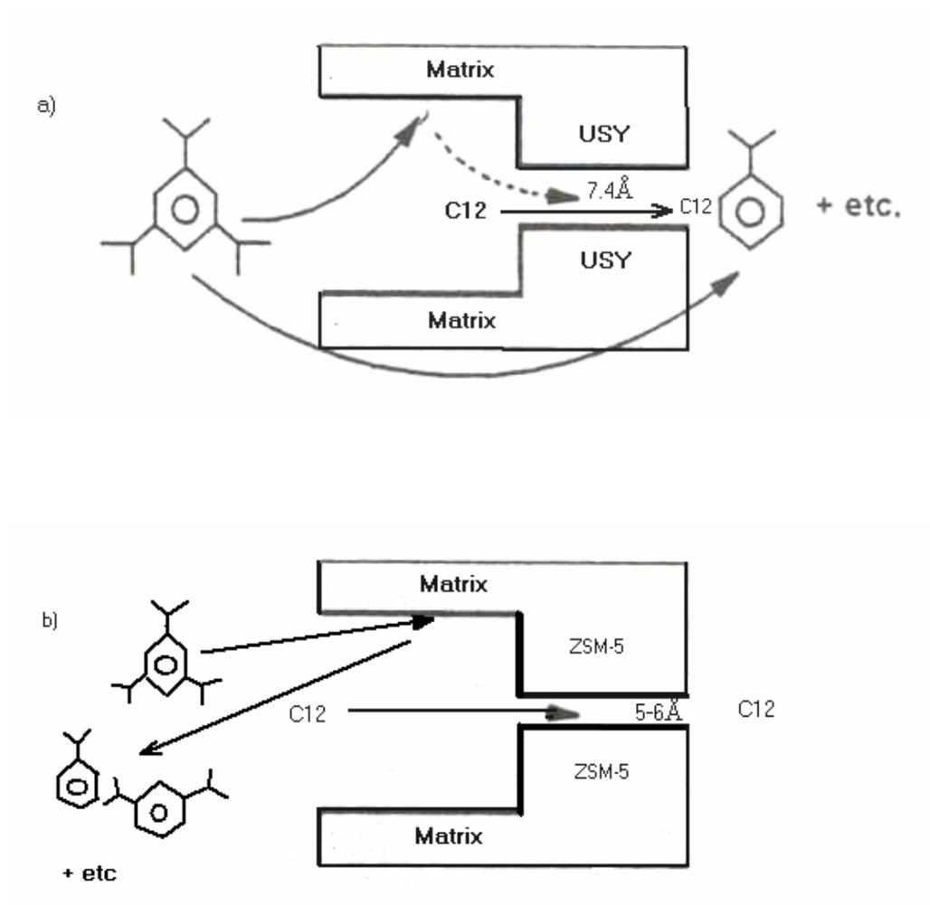
Figure 7: Effect of Pore Accessibility for 1,3,5-TIPB and n-dodecane cracking
