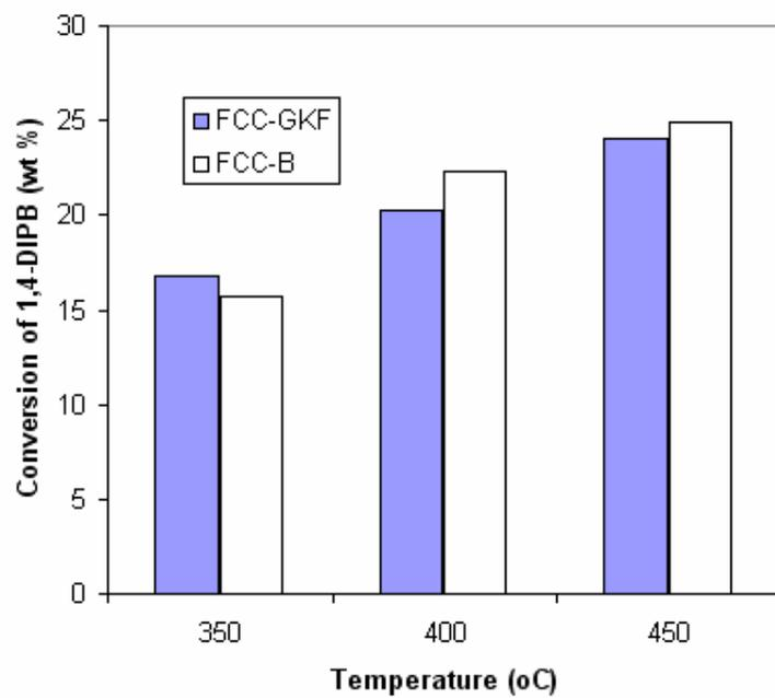
Figure 11: 1,4-DIPB conversion at 10-s reaction time and various temperatures
