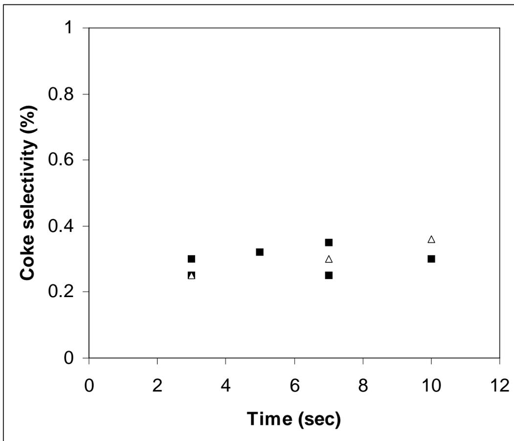
Figure 14. Coke selectivity for 1,3 5,-TIPB conversion versus reaction time. C/O=5, CAT-LC, (■) T=500°C, (△) T=550°C.
