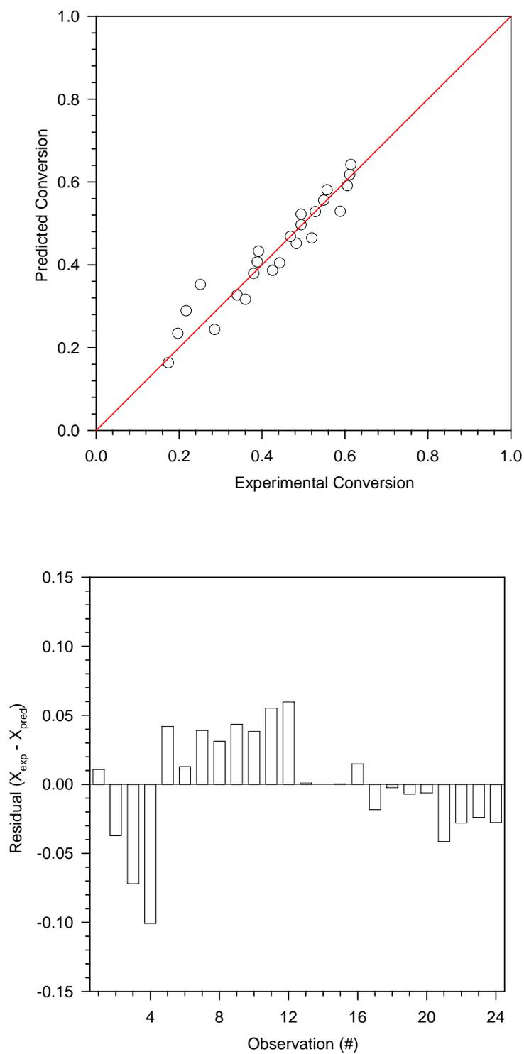
Figure 10b. Comparison between experimental data and RC model for the 1,3,5-TIPB conversion (CAT-SC).
