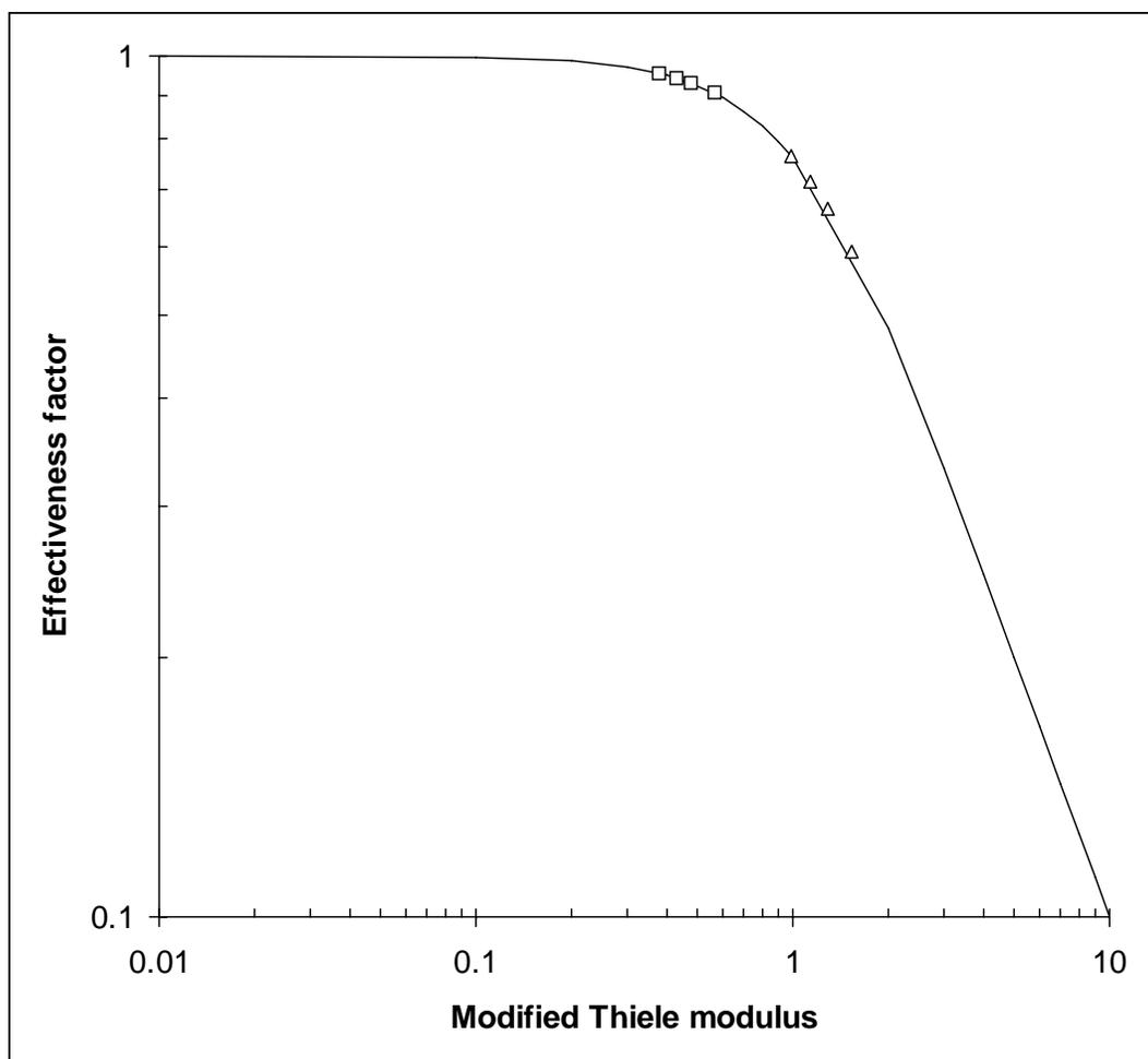
Figure 19. Effectiveness factor for 1,3,5-TIPB conversion versus modified Thiele modulus (RC model) for different reaction time.  $T=450^{\circ}\text{C}$ ,  $C/O=5$ . (□) CAT-SC, (△) CAT-LC.
