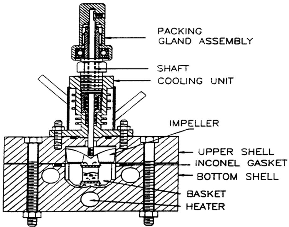
Figure 4. Schematic representation of CREC Riser Simulator.
