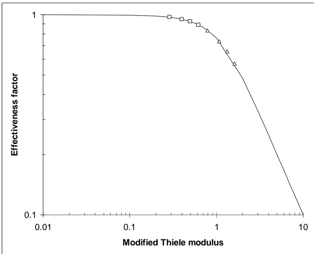
Figure 16. The effectiveness factor for the 1,3,5-TIPB conversion versus modified Thiele modulus (TOS model) for different reaction times.  $T=450^{\circ}\text{C}$ ,  $C/O=5$ , (□) CAT-SC, (△) CAT-LC
