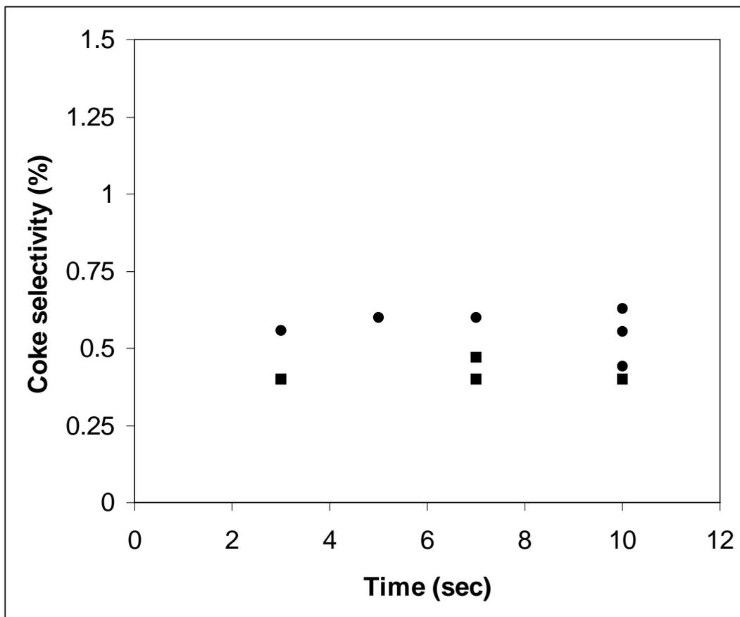
Figure 13. Coke selectivity for 1,3,5-TIPB conversion versus reaction time. C/O=5, CAT-LC, (●) T=400°C, (■) T=450°C.
