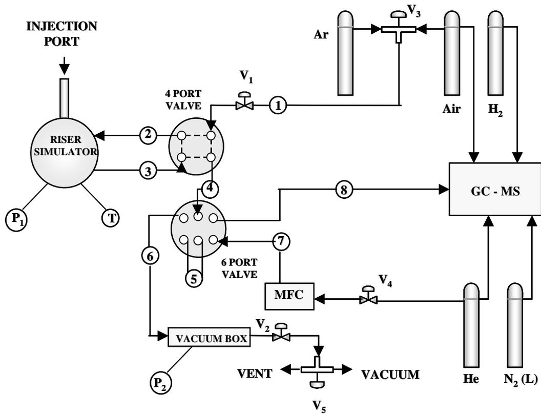
Figure 5. Schematic diagram of the Riser Simulator experimental setup and accessories.
