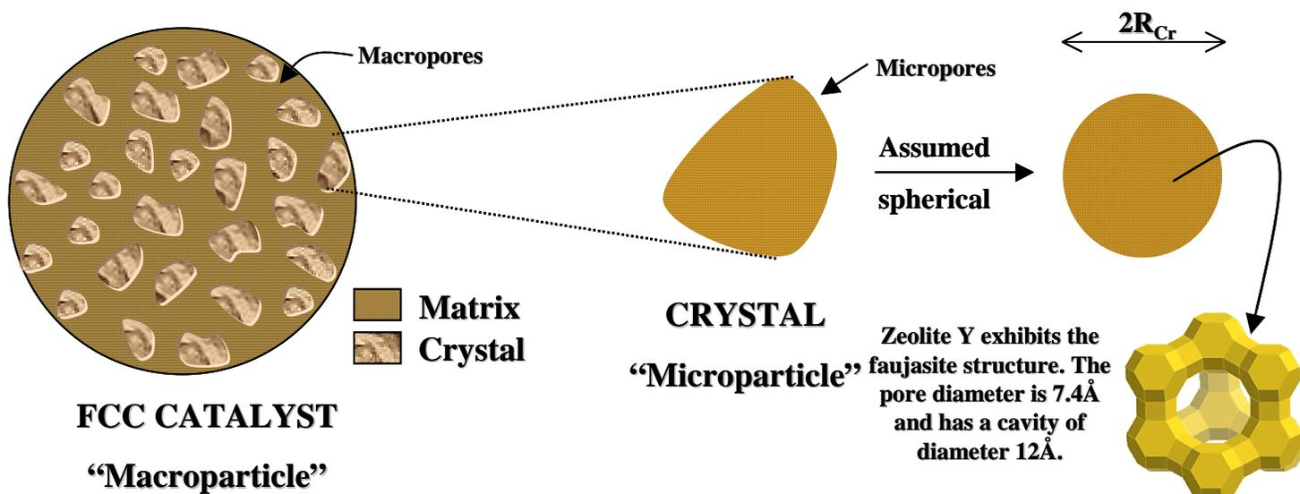
Figure 1. Configuration of an FCC catalyst pellet showing:
