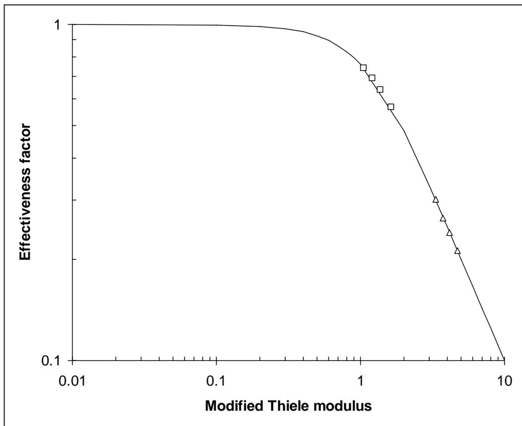
Figure 18. Effectiveness factor for 1,3,5-TIPB conversion versus modified Thiele modulus (RC model) for different reaction times.  $T=350^{\circ}\text{C}$ ,  $C/O=5$ . ( $\square$ ) CAT-SC, ( $\triangle$ )CAT-LC.
