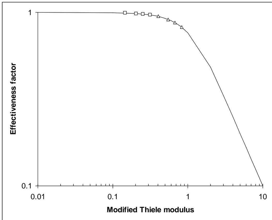
Figure 17. Effectiveness factor for 1,3,5-TIPB conversion versus modified Thiele modulus (TOS model) for different reaction times.  $T=550^{\circ}\text{C}$ ,  $C/O=5$ . ( $\square$ ) CAT-SC, ( $\triangle$ ) CAT-LC.
