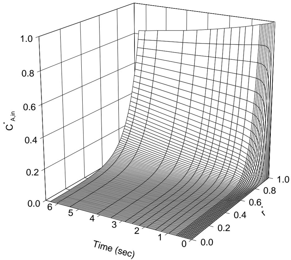
Figure 2. Changes of the dimensionless concentration with radial position inside the Y zeolite crystals between 0 and 6-sec. of reaction time.  $T= 350^{\circ}\text{C}$ .
