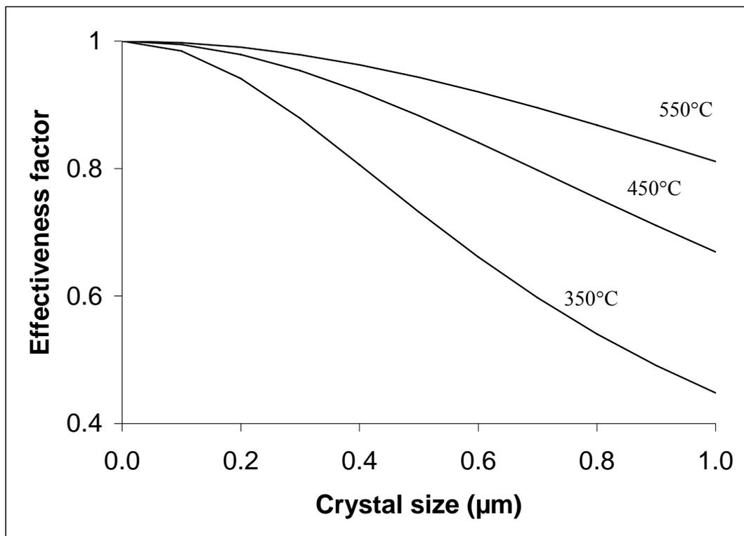
Figure 21. Effect of the zeolite crystal size on the effectiveness factor (RC-model).
