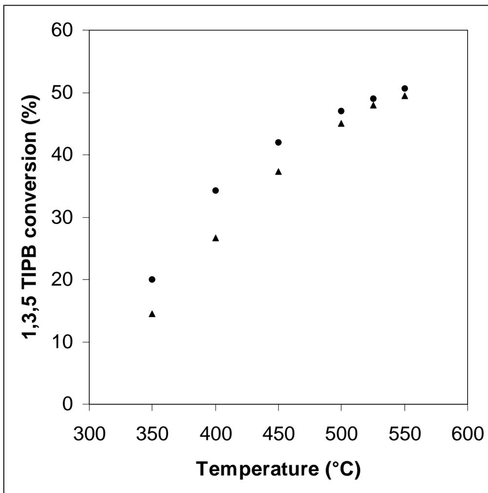
Figure 8. 1,3,5-TIPB cracking. Effect of temperature and Y-zeolite crystal size on 1,3,5-TIPB conversion. Reaction time =5 sec., C/O =5, (●) CAT-SC, (▲) CAT-LC.
