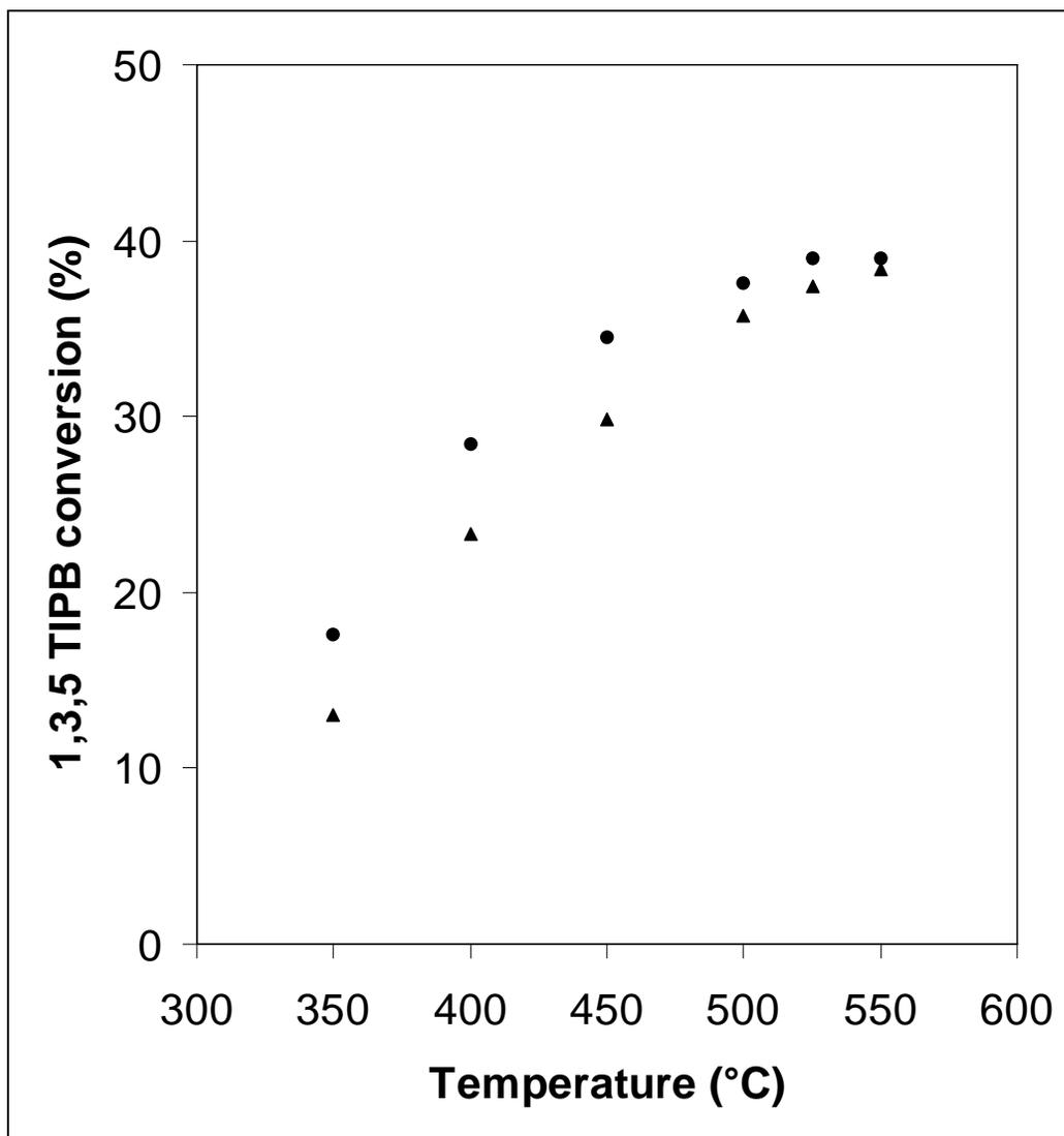
Figure 7. 1,3,5-TIPB cracking. Effect of temperature and Y-zeolite crystal size on 1,3,5-TIPB conversion. Reaction time =3 sec., C/O =5, (●) CAT-SC, (▲) CAT-LC. Reported experimental points are average values of at least 3 measurements.
