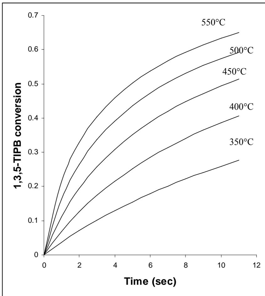
Figure 11. 1,3,5-TIPB conversion versus reaction time using RC model for CAT-LC, C/O=5.
