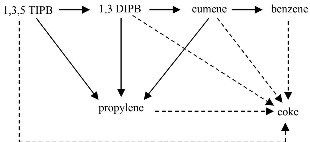
Figure 6. Schematic description of the catalytic cracking of 1,3,5-TIPB.
