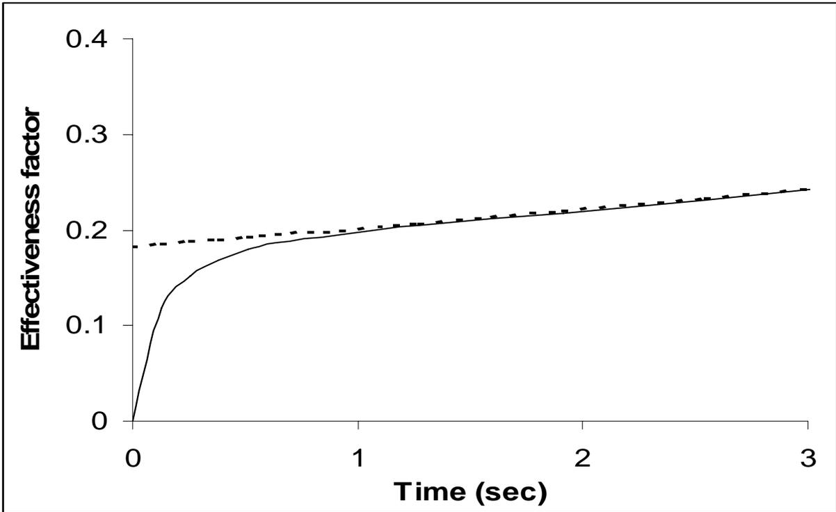
Figure 3a. Changes of the effectiveness factor with reaction time. Full line represents the calculated  $\eta$  values with eq(3) and the dimensionless concentration profiles given by eq(2). Broken line represents the calculated  $\eta_{ss}$  using the quasi-steady state approximation with the accumulation term of eq. (3) neglected.
