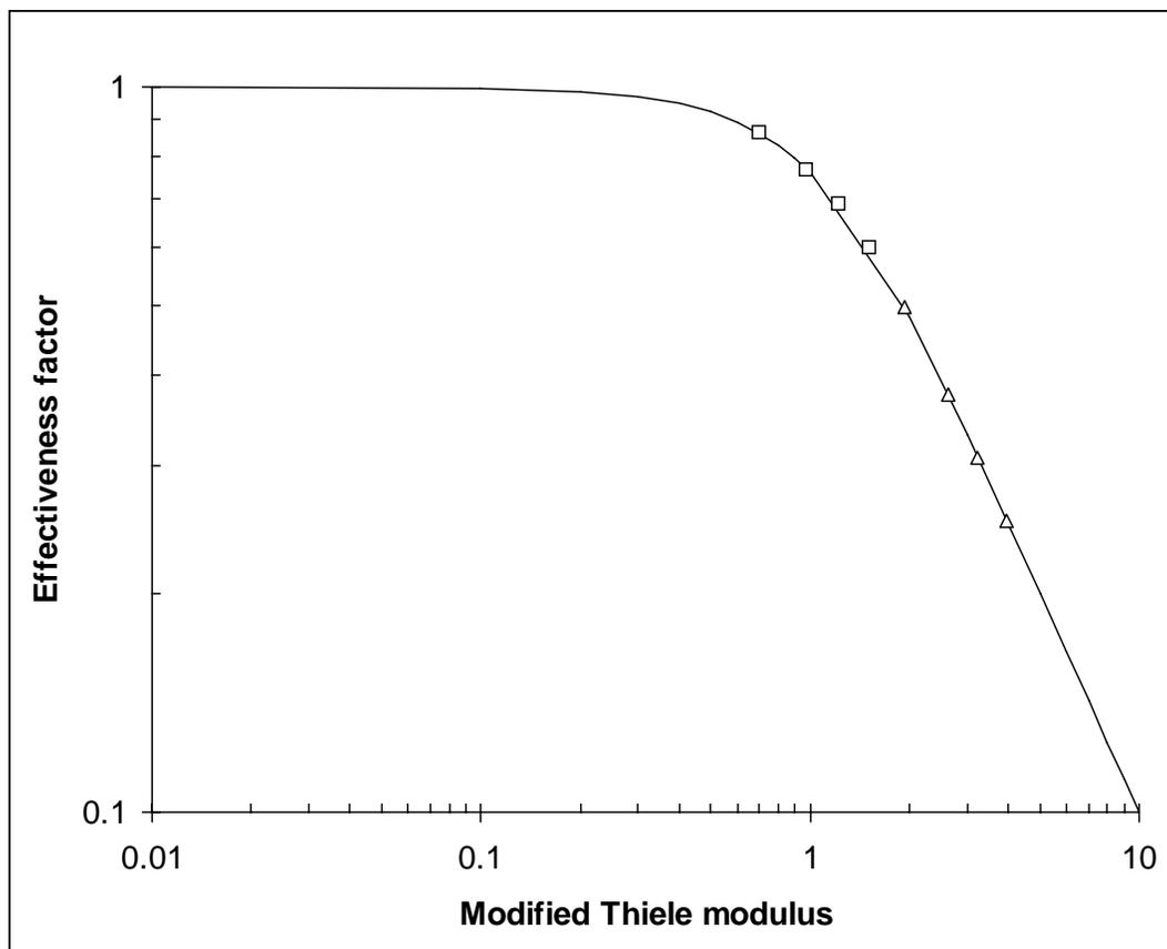
Figure 15. Effectiveness factor for the 1,3,5-TIPB conversion versus modified Thiele modulus (TOS model) for different reaction times.  $T=350^{\circ}\text{C}$ ,  $C/O=5$ , (□) CAT-SC, (△) CAT-LC.
