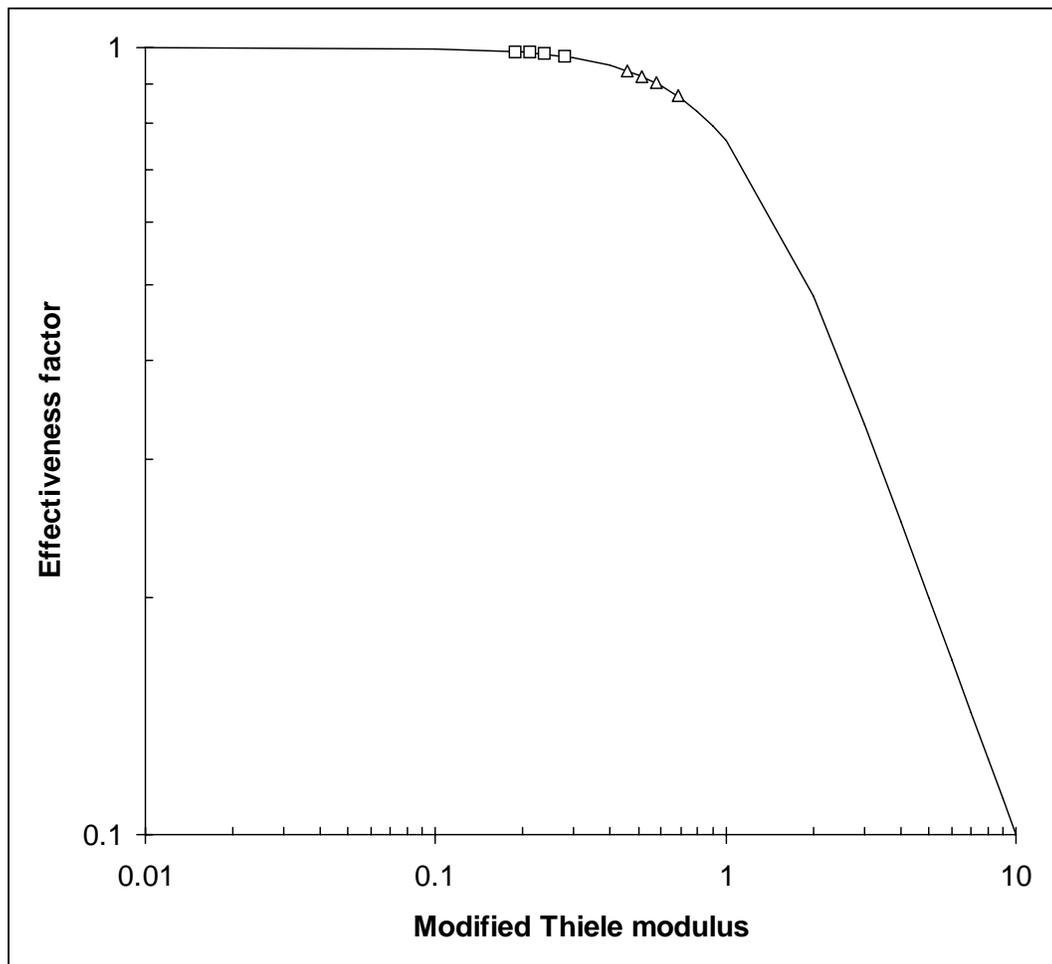
Figure 20. Effectiveness factor for 1,3,5-TIPB conversion versus modified Thiele modulus (RC model) for different reaction times.  $T=550^{\circ}\text{C}$ ,  $C/O=5$ . ( $\square$ ) CAT-SC, ( $\triangle$ ) CAT-LC.
