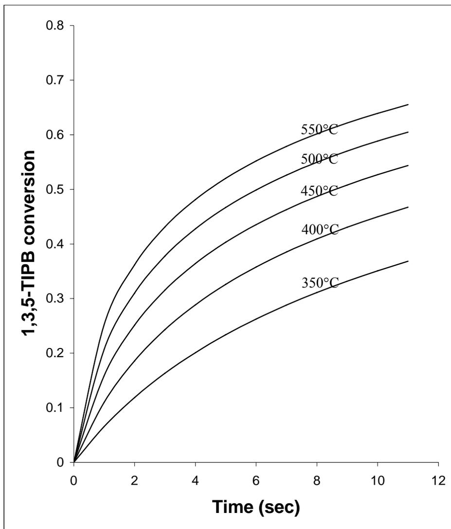
Figure 12. 1,3,5-TIPB conversion versus reaction time using RC model for CAT-SC, C/O=5.
