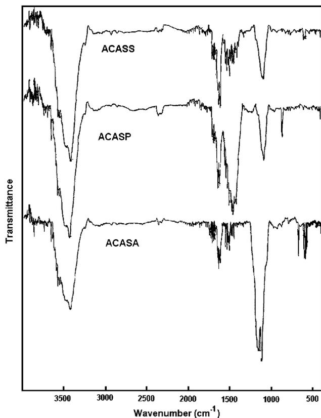
Fig. 1. FT-IR spectrum of activated carbo-aluminosilicate samples.
