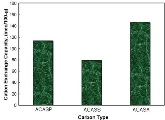
Fig. 5. Cation exchange capacity of activated carbo-aluminosilicate samples.
