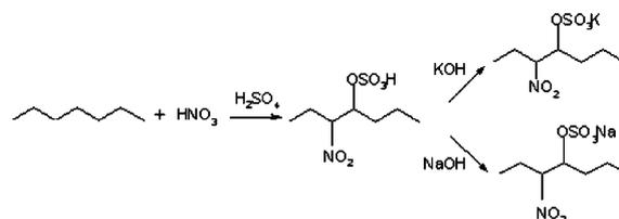
Scheme 1. Proposed chemical reaction of surface of oil shale with the activation agents.
