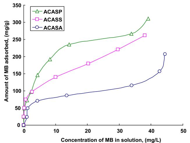
Fig. 6. Adsorption isotherms for the activated carbo-aluminosilicate samples.
