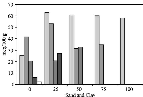
Fig. 7: Cation Exchange Capacity of Samples at Different Clay and Sand Ratios
