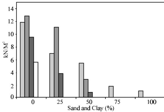
Fig. 3: Compressive Strength for Different Compositions of Sand-clay-cement Mixture Obtained after Three Weeks of Molding
