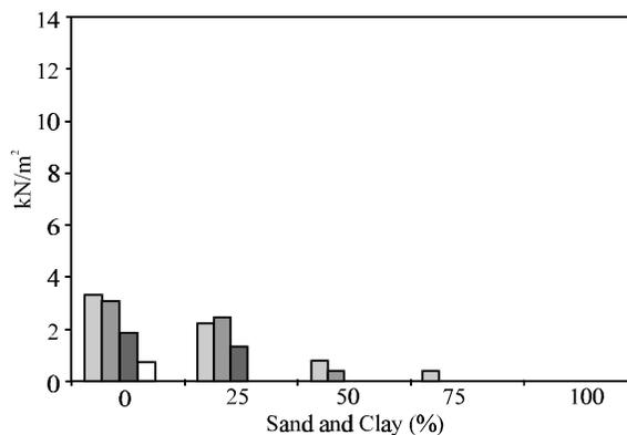
Fig. 1: Compressive Strength for Different Compositions of Sand-clay-cement Mixture Obtained after One Day of Molding
