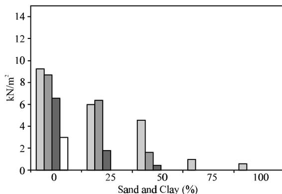
Fig. 2: Compressive Strength for Different Compositions of Sand-clay-cement Mixture Obtained after One Week of Molding
