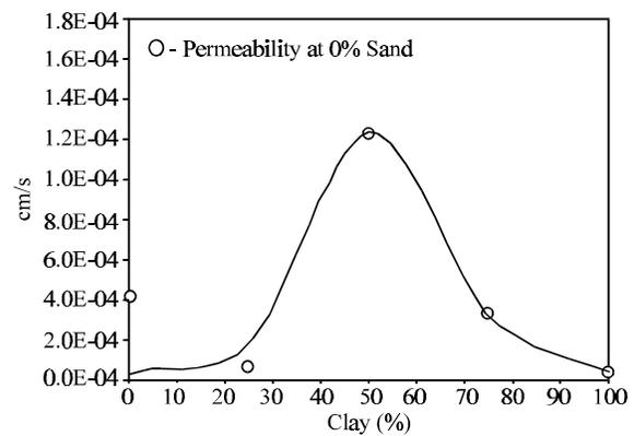
Fig. 6: Effect of Variation of Clay to Cement on the Permeability of the Mixture
