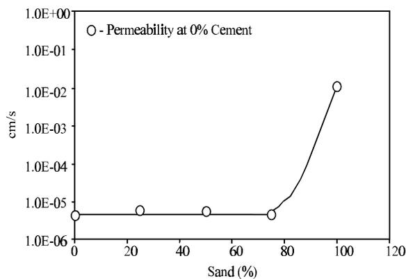
Fig. 4: Effect of Variation of Sand to Clay Ratio on Permeability of the Mixture
