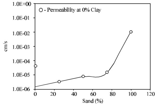
Fig. 5: Effect of Variation of Sand to Cement Ratio on the Permeability of the Mixture
