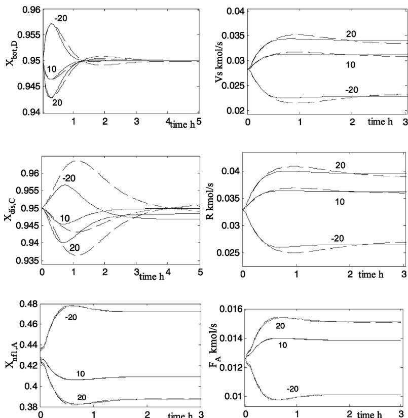
Figure 9. Single-end composition control responses,  $-20\%$ ,  $+10\%$ , and  $+20\%$   $F_B$ : (---) linear model; (—) nonlinear model.
