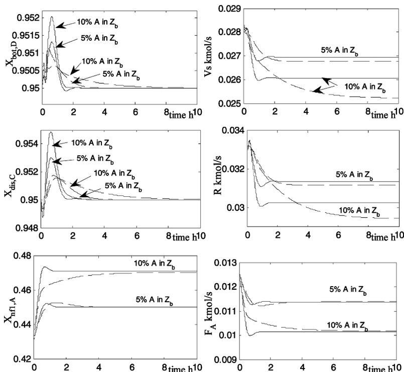
**Figure 4.** Dual-end composition control responses, 5% and 10% mol of reactant A in  $Z_b$ : (---) linear model; (—) nonlinear model.
