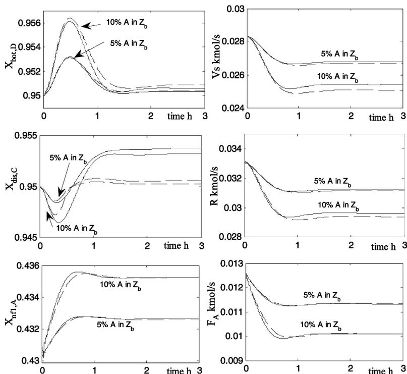
Figure 14. Single-end temperature control responses, 5% and 10% mol of reactant A in  $Z_b$ : (---) linear model; (—) nonlinear model.
