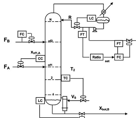
**Figure 12.** Single-end temperature control structure.
