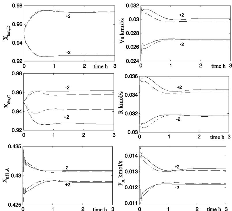
**Figure 15.** Single-end temperature control responses,  $\pm 2$  K changes in temperature on tray 2: (---) linear model; (—) nonlinear model.
