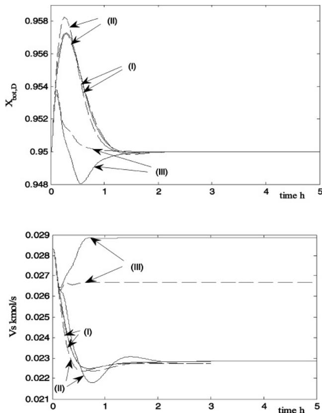
**Figure 6.** Three alternative control schemes for a single-end control structure: (I) fixed reflux ratio and control level by the reflux flow rate; (II) fixed reflux ratio and control level by the distillate flow rate ( $D$ ); (III) fixed reflux flow rate and control level by the distillate flow rate.
