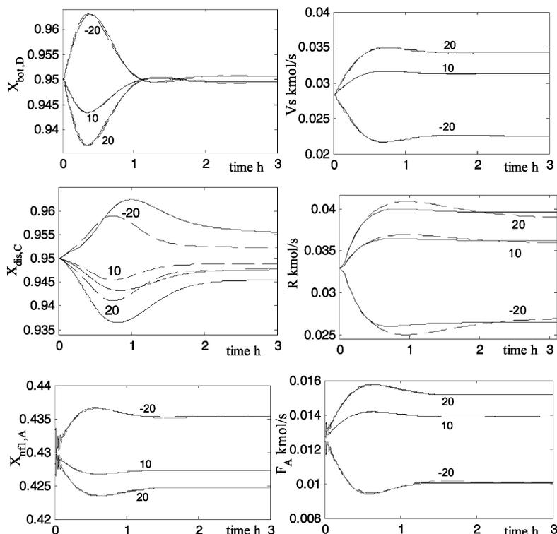
Figure 13. Single-end temperature control responses,  $-20\%$ ,  $+10\%$ , and  $+20\%$   $F_B$ : (---) linear model; (—) nonlinear model.
