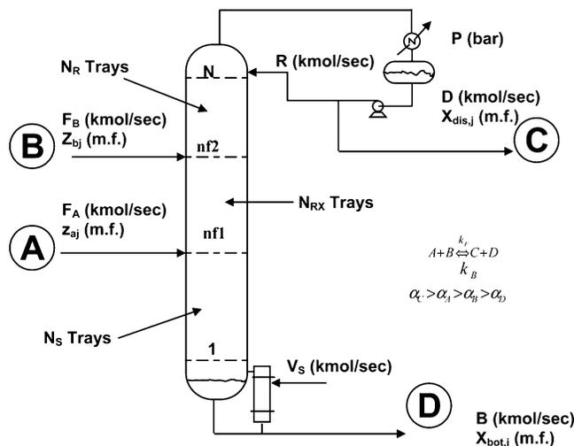
Figure 1. Reactive distillation column.
