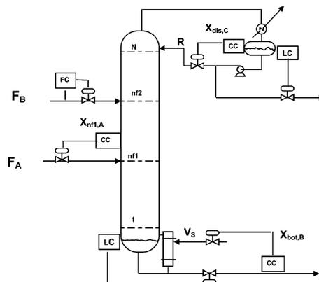
Figure 2. Dual-end composition control structure.
