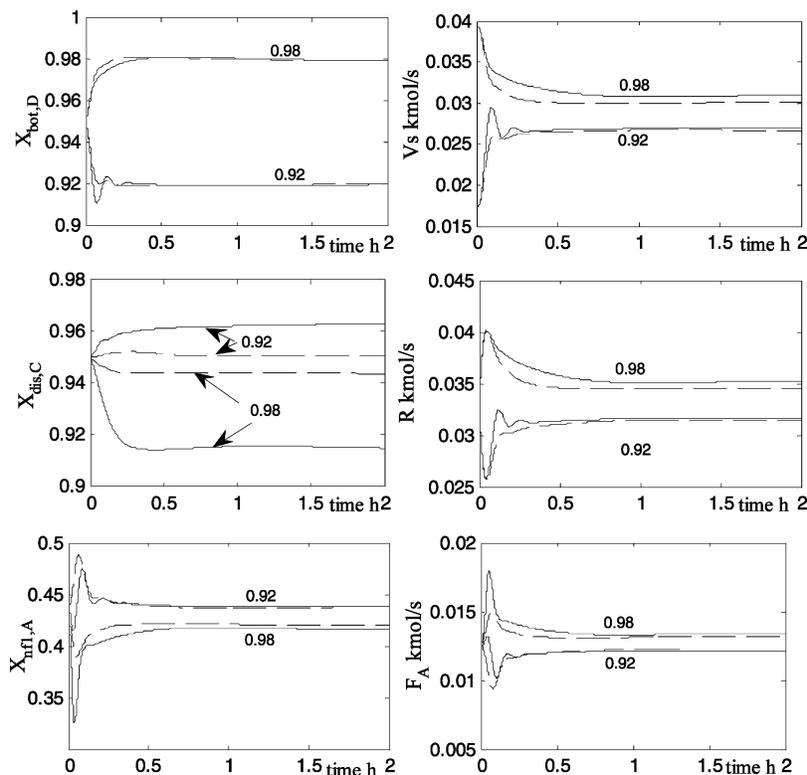
**Figure 11.** Single-end composition control responses, setpoint changes  $X_{bot,B}$  from 95% to 92% and 98%: (---) linear model; (—) nonlinear model.
