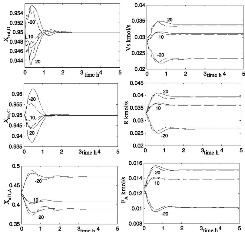
**Figure 3.** Dual-end composition control responses,  $-20\%$ ,  $+10\%$ , and  $+20\%$   $F_B$ : (---) linear model; (—) nonlinear model.
