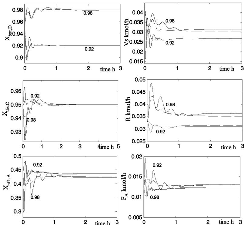
**Figure 5.** Dual-end composition control responses, setpoint changes  $X_{bot,B}$  from 95% to 92% and 98%: (---) linear model; (—) nonlinear model.
