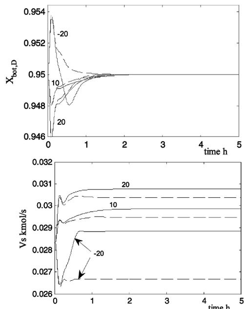
**Figure 7.** Single-end composition control responses based on scheme 3 with -20%, +10%, and +20% disturbances in  $F_B$ : (---) linear model; (—) nonlinear model.
