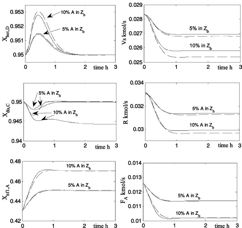
Figure 10. Single-end composition control responses, 5% and 10% mol of A in  $Z_b$ : (---) linear model; (—) nonlinear model.
