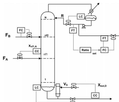
**Figure 8.** Single-end composition control structure.
