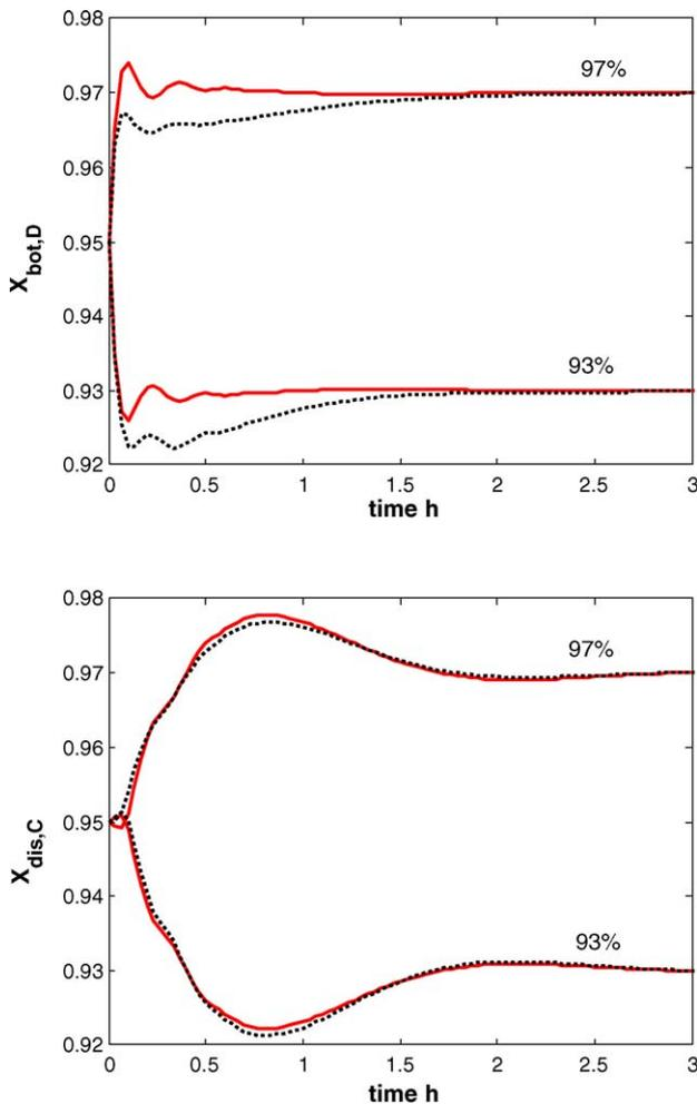
Fig. 8. Control performance to setpoint changes:  $x_{bot,D}$  and  $x_{dis,C}$  from 95 to 93% and to 97%; the base initial conditions error,  $\delta_m = 10\%$  and  $\delta_p = 1\%$  are used for KF design; (—) measured states for feedback; (---) estimated states for feedback.
