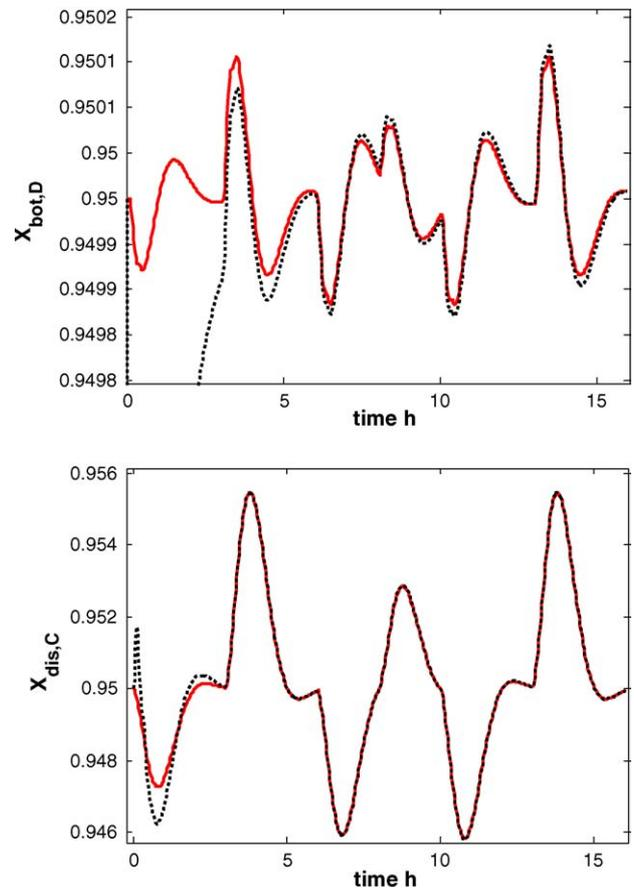
Fig. 7. Control performance with a PRRS forcing function on  $F_B$ . The base initial condition errors,  $\delta_m = 10\%$  and  $\delta_p = 1\%$  are used for KF design. (—) measured states for feedback; (---) estimated states for feedback.
