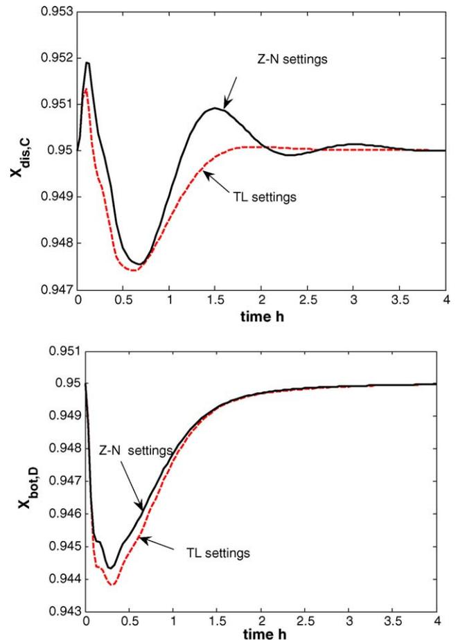
Fig. 5. Effect of tuning methods on the performance of estimator-based controllers with a disturbance of 10%  $F_B$ : (—) TL tuning; (---) Z–N tuning.
