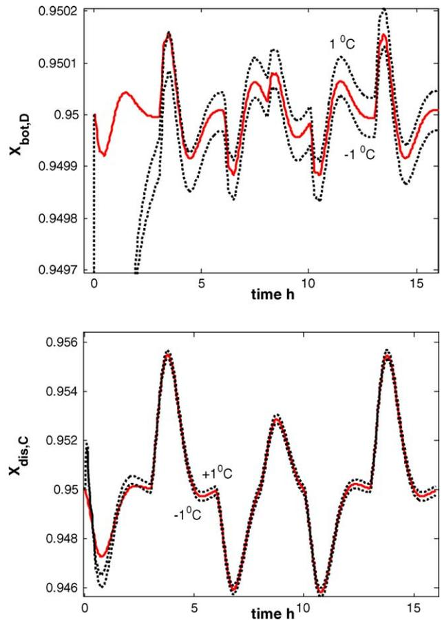
Fig. 10. Effect of erroneous relative volatility on control performance with a PRRS forcing function on  $F_B$ : the base initial conditions error,  $\delta_m = 10\%$  and  $\delta_p = 1\%$  are used for KF design; (—) measured states for feedback; (---) estimated states for feedback.
