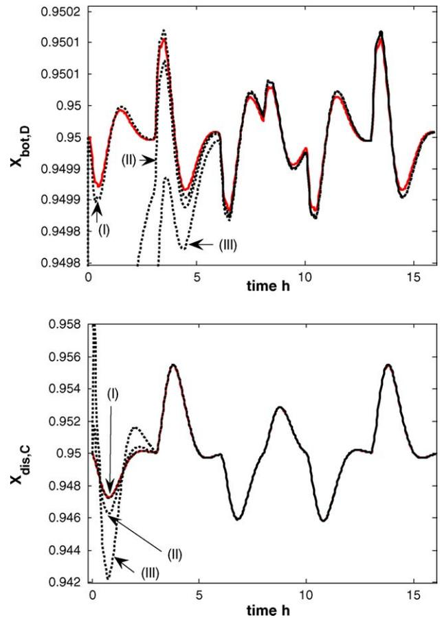
Fig. 9. Effect of erroneous initial conditions on the control performance with a PRRS forcing function on  $F_B$ : (I) no error; (II) base error ( $X_0$  err); (III)  $5X_0$  err,  $\delta_m = 10\%$  and  $\delta_p = 1\%$  are used for KF design, (—) measured states for feedback; (---) estimated states for feedback.
