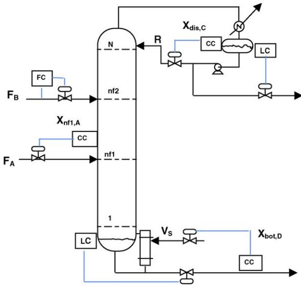
Fig. 3. Dual-end composition control structure.
