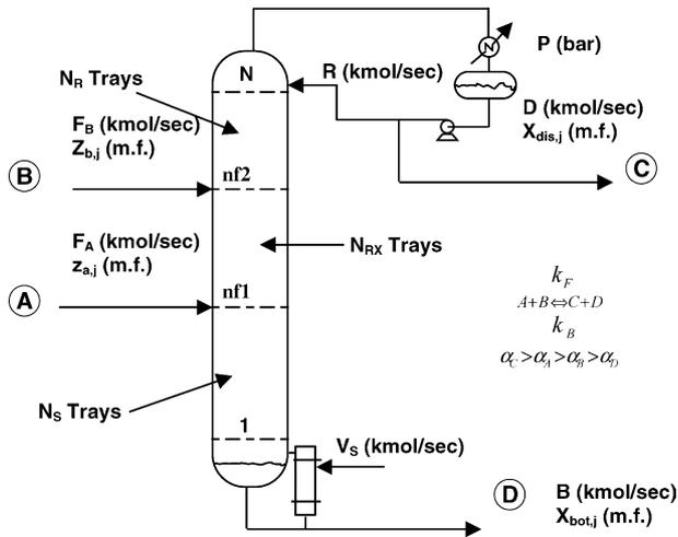
Fig. 1. Reactive distillation column.
