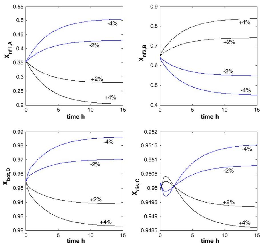
Fig. 2. Dynamic composition profile of the reactant A on the tray  $nf_1$ , the reactant B on the tray  $nf_2$ , the product C in the distillate and the product D in the bottoms with  $\pm 2$  and  $\pm 4\%$  change in  $F_B$ .
