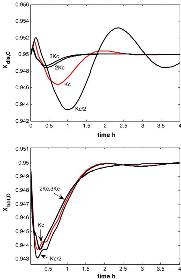
Fig. 6. Control performance at different values of controller gains with a disturbance of 10%  $F_B$ .  $K_c$  is the gain obtained from TL tuning.
