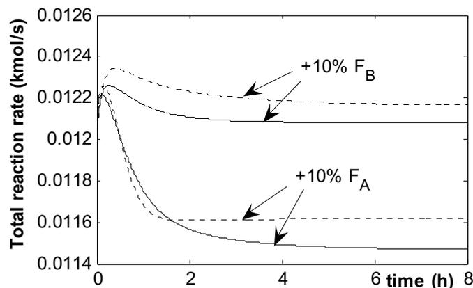
Figure 2. Dynamic responses of total reaction rate to positive step changes in feed flowrates of reactant A and B. (—) OL-I; (---) OL-II.
