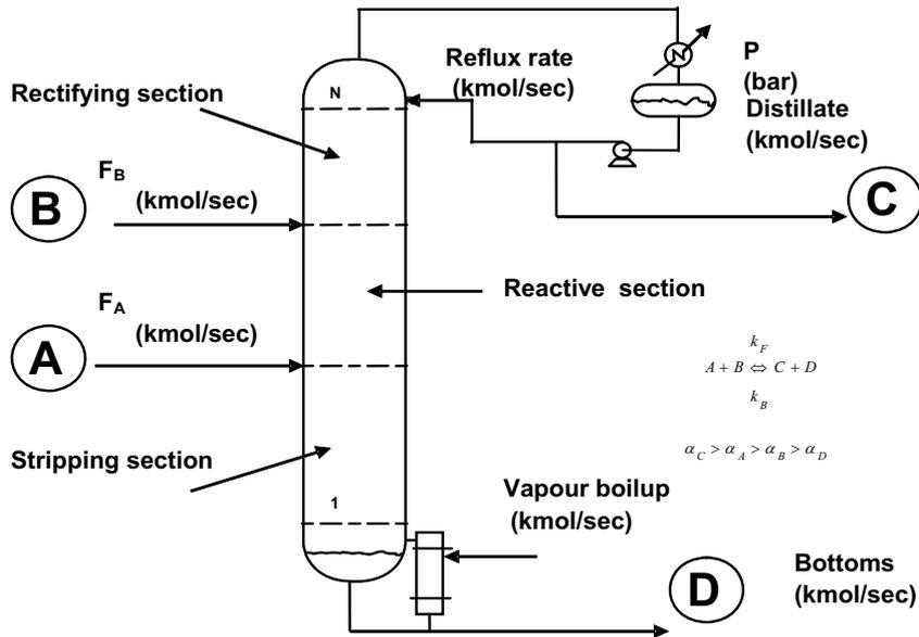
Figure 1. Distillation column
