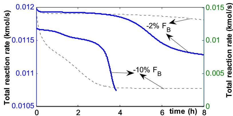
Figure 4. Dynamic responses of total reaction rate to negative step changes in feed flowrates of reactant A and B. (—) OL-I; (---) OL-II.
