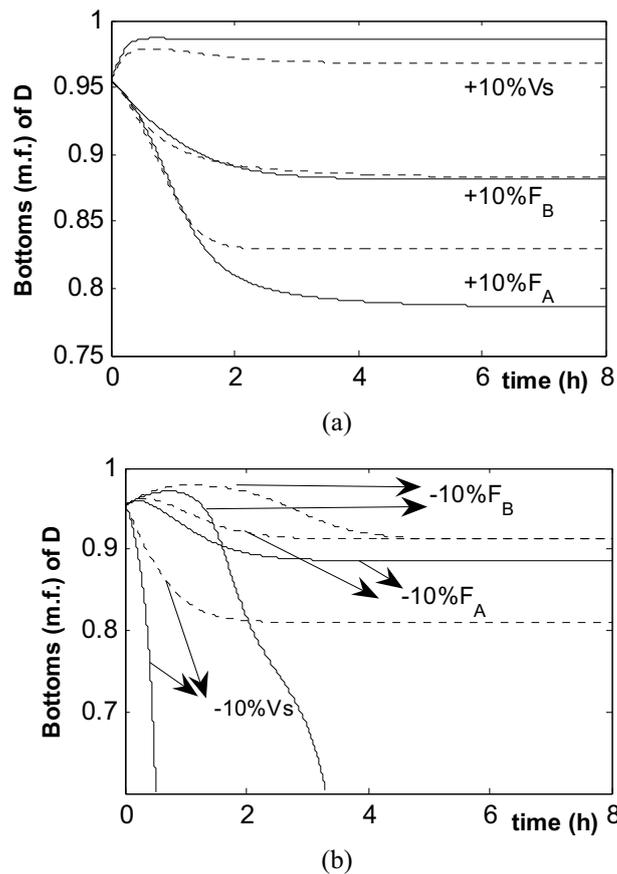
Figure 3. Composition dynamic responses of product D in bottoms to step changes in feed flowrate of reactant A ( $F_A$ ), feed flowrate of B ( $F_B$ ) and vapor boilup ( $V_s$ ).
