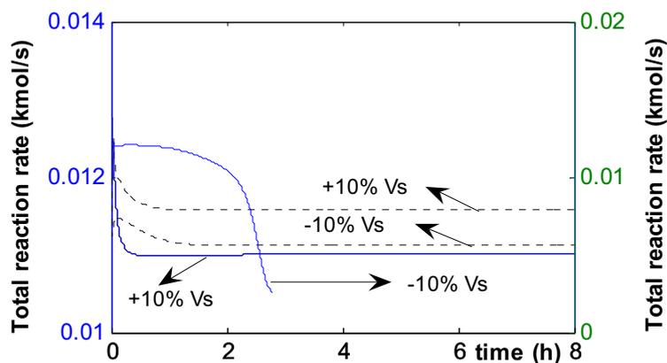
Figure 5. Dynamic responses of total reaction rate to step changes in vapor boilup ( $V_s$ ) (—) OL-I; (---) OL-II.
