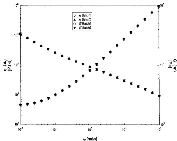
Fig. 1. Reproducibility test.  $\eta'(\omega)$  and  $G'(\omega)$  for 50/50 blend ( $T_{test} = 190^\circ\text{C}$ ,  $\gamma^o = 15\%$ ).
