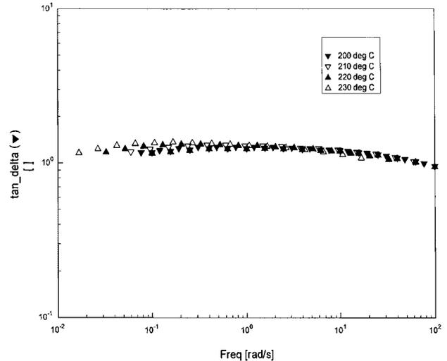
Fig. 5. Master curve for 90% HNBR blend. ( $T_{test} = 190^\circ\text{C}$ ,  $\gamma^\circ = 15\%$ ,  $T_{range} = 200^\circ\text{C} - 230^\circ\text{C}$ ).
