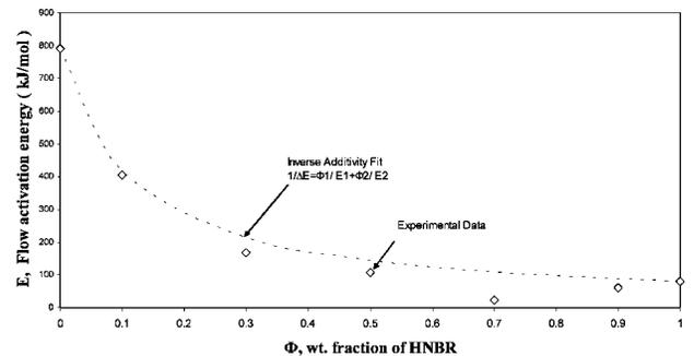
Fig. 6. Flow activation energy vs. weight fraction ( $\phi$ ) of HNBR.
