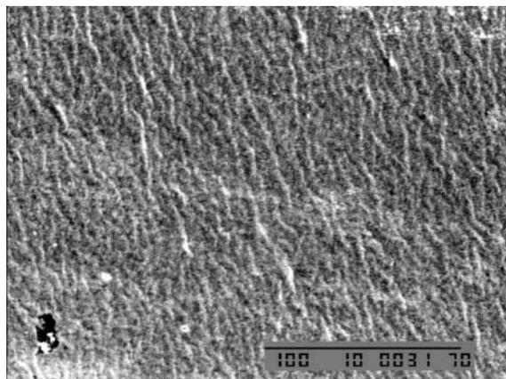
Fig. 7c. SEM micrographs for 90/10 HNBR/NBR blends.
