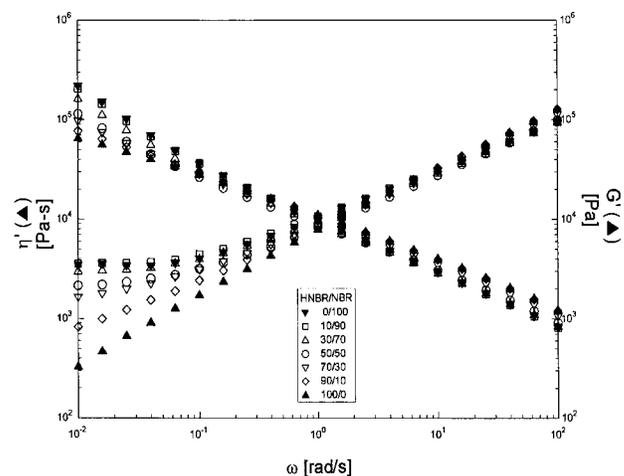
Fig. 2.  $\eta'(\omega)$  and  $G'(\omega)$  for blends, as well as the pure samples ( $T_{test} = 190^\circ\text{C}$ ,  $\gamma^o = 15\%$ ).
