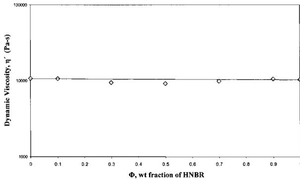
Fig. 4a. Dynamic viscosity  $\eta'(\phi)$  as a function of weight fraction of HNBR. ( $\omega = 0.03$ ) (—) linear rule of mixture.
