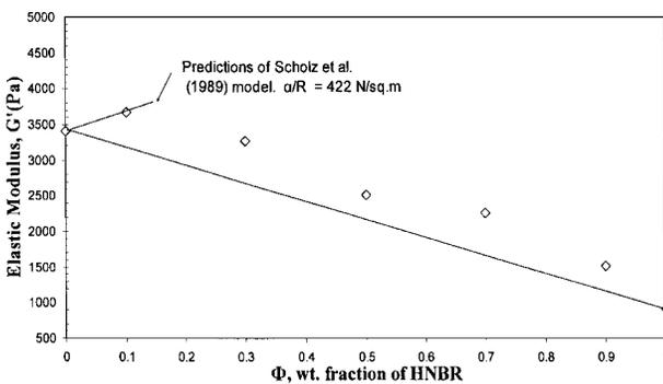
Fig. 4b. Elastic modulus  $G'(\phi)$  as a function of weight fraction of HNBR ( $\omega = 0.03$ ) (—) linear rule of mixture.
