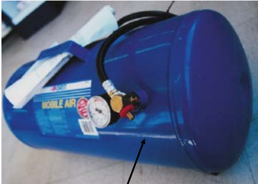
Pressurized tank (photo courtesy P.M. Anderson)
