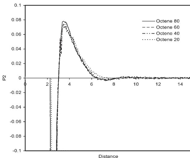
**Figure 3.** Intermolecular orientation correlation function for the PE with different branch.
