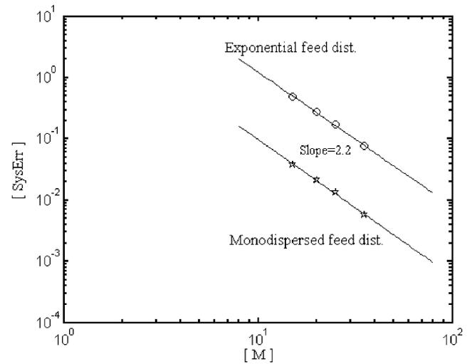
Fig. 17. The convergence characteristics of the moving pivot technique for droplet breakage in a continuous vessel with  $\Gamma = v$  and  $\beta(v|v) = 1/v$ , binary breakage, and  $\tau = 5$ .
