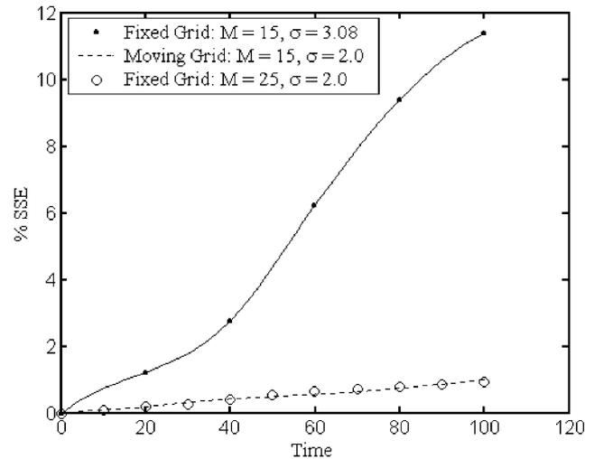
Fig. 8. The effect of the approximate optimal and fixed grids on the SSE using different levels of discretization for droplet breakage in a batch vessel with binary breakage,  $\Gamma = v^2$ ,  $\beta(v|v) = 1/v$ , and exponential initial condition.
