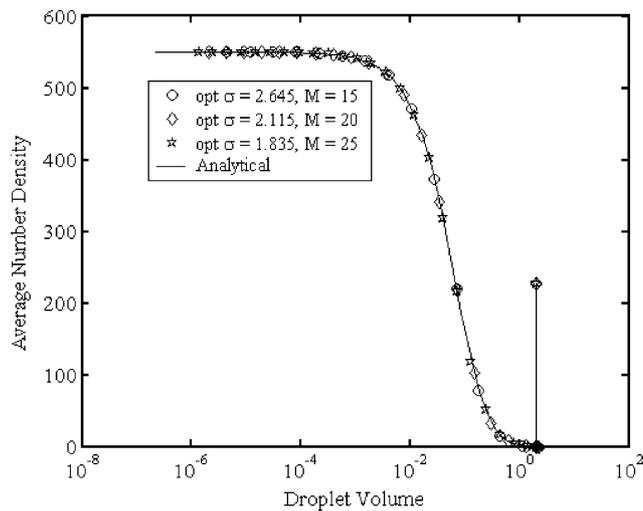
Fig. 15. Effect of the optimal geometric grid factor on the steady-state number density for droplet breakage in a continuous vessel with  $\Gamma = v$  and  $\beta(v|v) = 1/v$ , binary breakage,  $\tau = 5$ , and monodisperse feed distribution.
