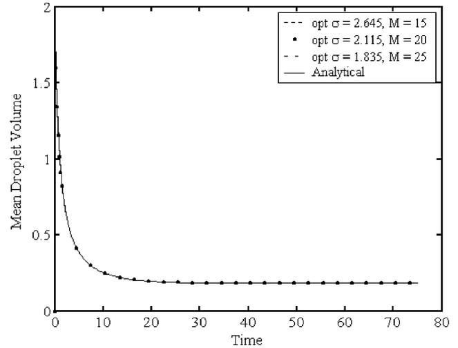
Fig. 16. Effect of the optimal geometric grid factor on the mean droplet volume for droplet breakage in a continuous vessel with  $\Gamma = v$  and  $\beta(v|v) = 1/v$ , binary breakage,  $\tau = 5$ , and monodisperse feed distribution.
