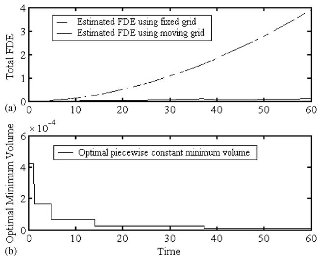
Fig. 9. (a) The effect of the optimal grid movement on the total FDE. (b) The approximate optimal minimum droplet volume profiles for droplet breakage in a batch vessel using a geometric grid with factor  $\sigma = 2.5$ ,  $M = 12$ , binary breakage,  $\Gamma = v$ ,  $\beta(v|v')$  = parabolic, and exponential initial condition.
