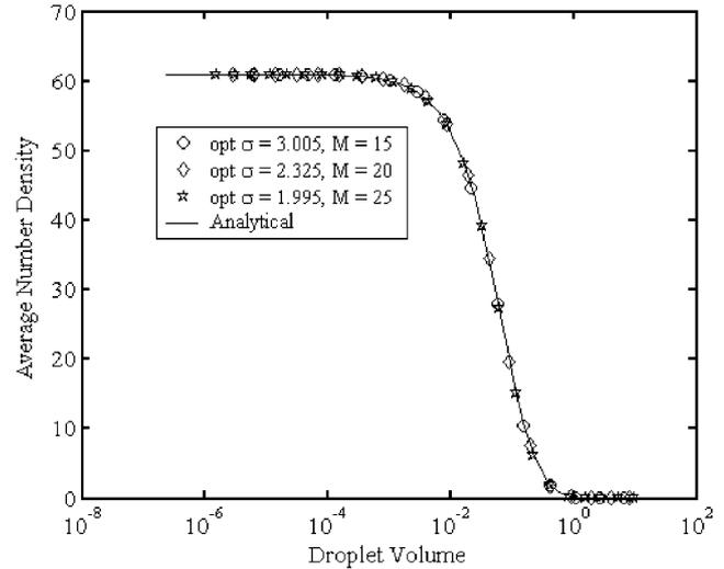
Fig. 12. Effect of the optimal geometric grid factor on the steady-state number density for droplet breakage in a continuous vessel with  $\Gamma = v$  and  $\beta(v|v) = 1/v$ , binary breakage,  $\tau = 5$ , and exponential feed distribution.
