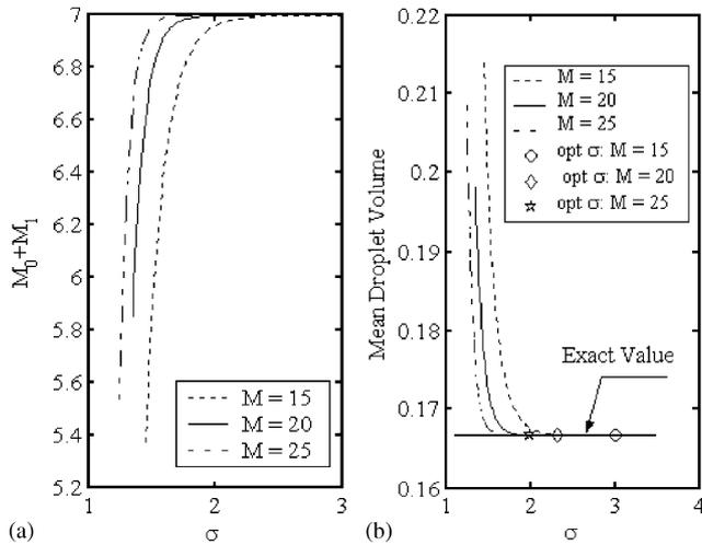
Fig. 11. Effect of the optimal geometric grid factor on: (a) The steady-state sum of zero and first moments of the distribution. (b) The mean droplet volume for droplet breakage in a continuous vessel with  $\Gamma = v$  and  $\beta(v|v) = 1/v$ , binary breakage,  $\tau = 5$ , and exponential feed distribution.
