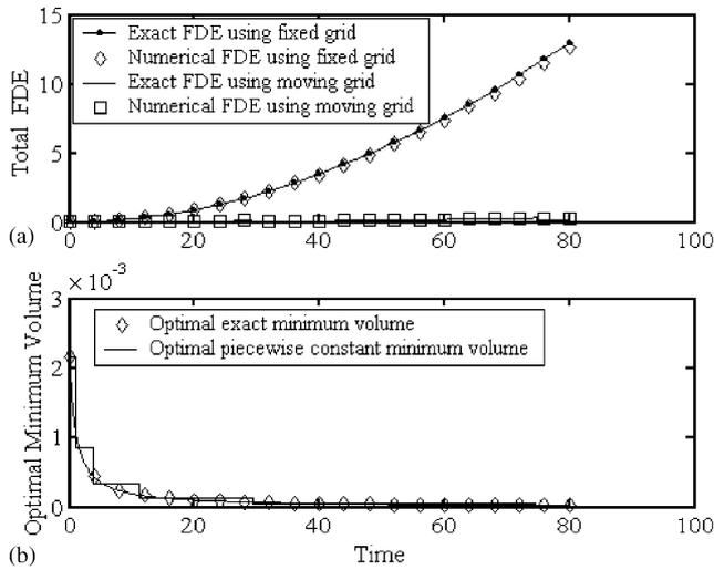
Fig. 2. (a) The effect of the optimal grid movement on the total FDE. (b) The approximate and exact optimal minimum droplet volume profiles for droplet breakage in a batch vessel using a geometric grid with factor  $\sigma = 2.5$ ,  $M = 10$ , binary breakage,  $\Gamma = v$ ,  $\beta(v|v) = 1/v$ , and exponential initial condition.
