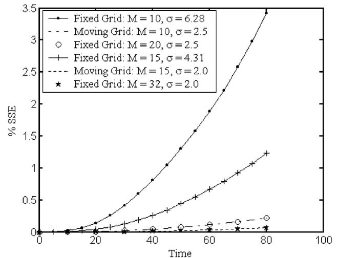
Fig. 4. The effect of the approximate optimal and fixed grids on the SSE using different levels of discretization for droplet breakage in a batch vessel with binary breakage,  $\Gamma = v$ ,  $\beta(v|v) = 1/v$ , and exponential initial condition.
