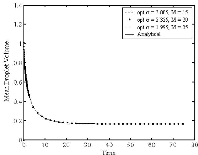
Fig. 13. Effect of the optimal geometric grid factor on the mean droplet volume for droplet breakage in a continuous vessel with  $\Gamma = v$  and  $\beta(v|v') = 1/v'$ , binary breakage,  $\tau = 5$ , and exponential feed distribution.
