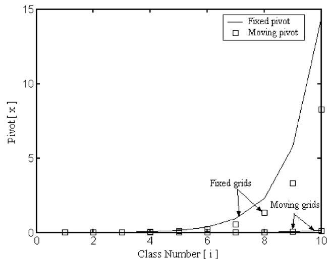
Fig. 5. The effect of the approximate optimal and fixed grids on the fixed and moving pivots at  $t = 80$  using a geometric grid with factor  $\sigma = 2.5$ ,  $M = 10$  for droplet breakage in a batch vessel with binary breakage,  $\Gamma = v$ ,  $\beta(v|v) = 1/v$ , and exponential initial condition.
