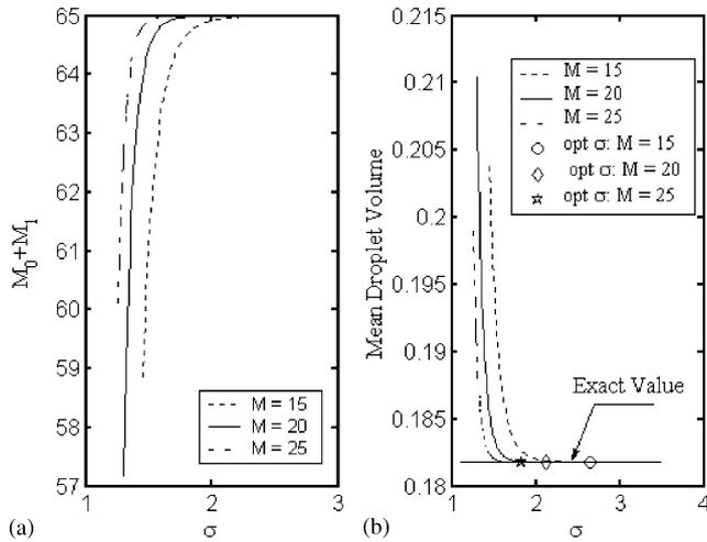
Fig. 14. Effect of the optimal geometric grid factor on: (a) The steady-state sum of zero and first moments of the distribution. (b) The mean droplet volume for droplet breakage in a continuous vessel with  $\Gamma = v$ ,  $\beta(v|v) = 1/v$ , binary breakage,  $\tau = 5$ , and monodisperse feed distribution.
