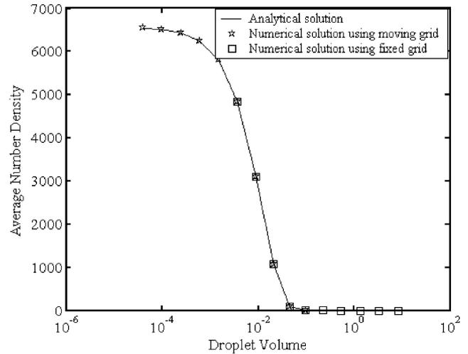
Fig. 3. The effect of the optimal grid movement on the average number density for droplet breakage in a batch vessel using a geometric grid with factor  $\sigma = 2.5$ ,  $M = 10$ , binary breakage,  $\Gamma = v$ ,  $\beta(v|v) = 1/v$ , exponential initial condition, and  $t = 80$ .
