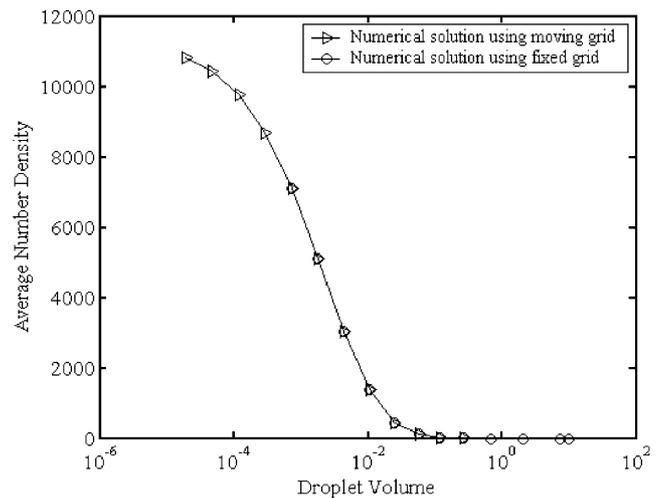
Fig. 10. The effect of the optimal grid movement on the average number density for droplet breakage in a batch vessel using a geometric grid with factor  $\sigma = 2.5$ ,  $M = 12$ , binary breakage,  $\Gamma = v$ ,  $\beta(v|v')$  = parabolic, and exponential initial condition.
