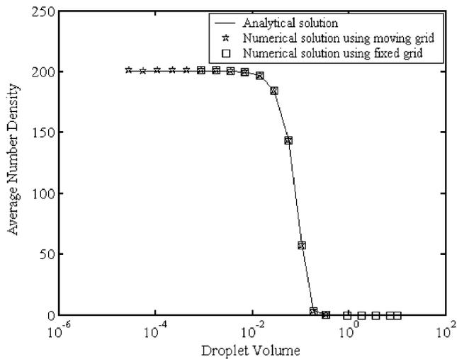
Fig. 7. The effect of the optimal grid movement on the average number density for droplet breakage in a batch vessel using a geometric grid with factor  $\sigma = 2$ ,  $M = 15$ , binary breakage,  $\Gamma = v^2$ ,  $\beta(v|v) = 1/v$ , and exponential initial condition.
