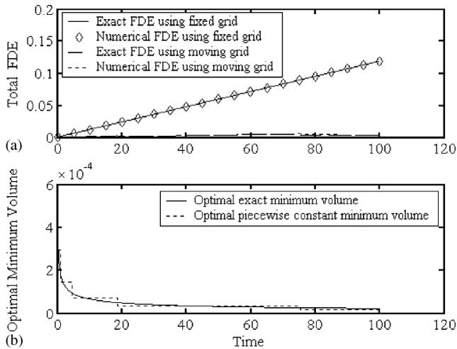
Fig. 6. (a) The effect of the optimal grid movement on the total FDE. (b) The approximate and exact optimal minimum droplet volume profiles for droplet breakage in a batch vessel using a geometric grid with factor  $\sigma = 2$ ,  $M = 15$ , binary breakage,  $\Gamma = v^2$ ,  $\beta(v|v) = 1/v$ , and exponential initial condition.
