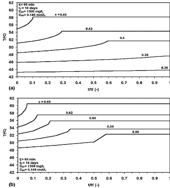
Fig. 9: Temperature profiles of an immobilized mesophilic lactose hydrolysis (a) CSTR, (b) PFR at different initial conversions and operating period of 16 days at a residence time of 60 min.
