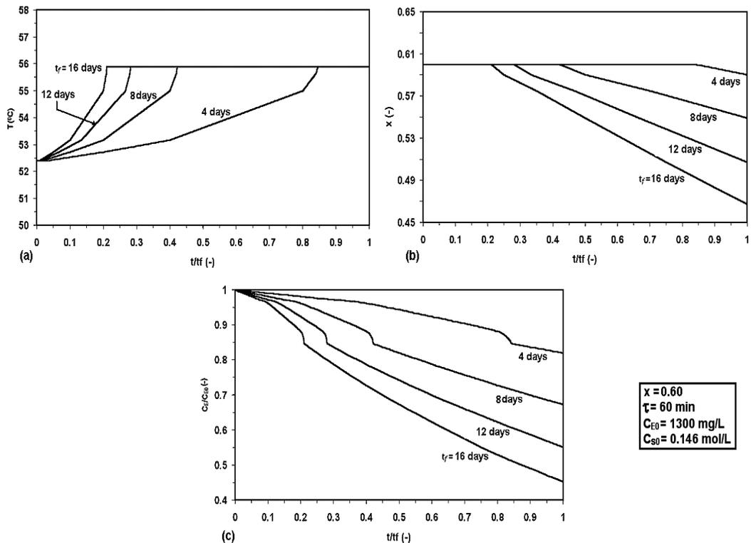
Fig. 2: (a) Temperature profiles, (b) Conversion profiles, (c) Activity profiles of an immobilized mesophilic lactose hydrolysis PFR at different operating periods, residence time of 60 min and enzyme concentration of 1300 mg/L.
