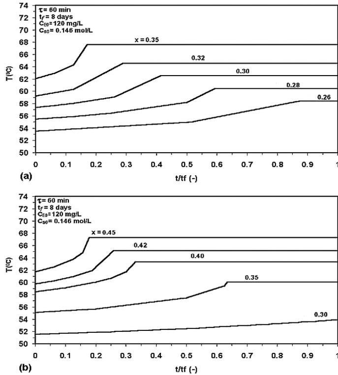
Fig. 10: Temperature profiles of an immobilized thermophilic lactose hydrolysis (a) CSTR, (b) PFR at different initial conversions and operating period of 8 days at a residence time of 60 min.
