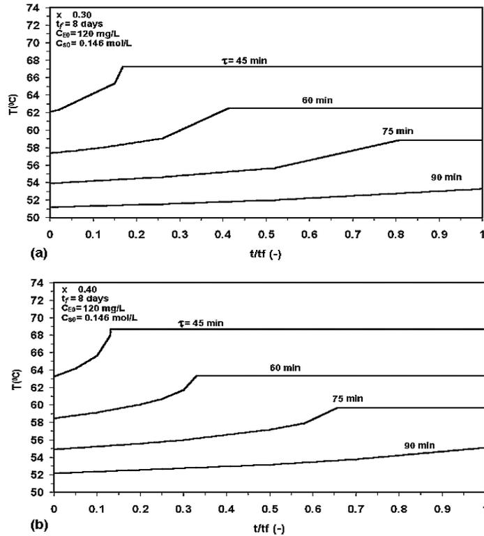
Fig. 6: Temperature profiles of an immobilized thermophilic lactose hydrolysis (a) CSTR, (b) PFR at different residence times and operating period of 8 days at enzyme concentration of 120mg/L.
