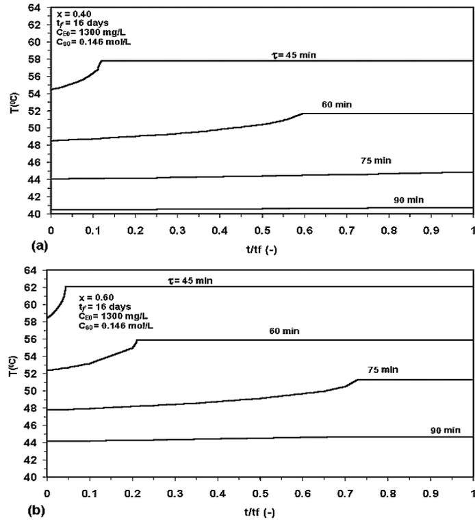
Fig. 5: Temperature profiles of an immobilized mesophilic lactose hydrolysis (a) CSTR, (b) PFR at different residence times and operating period of 16 days at enzyme concentration of 1300mg/L.
