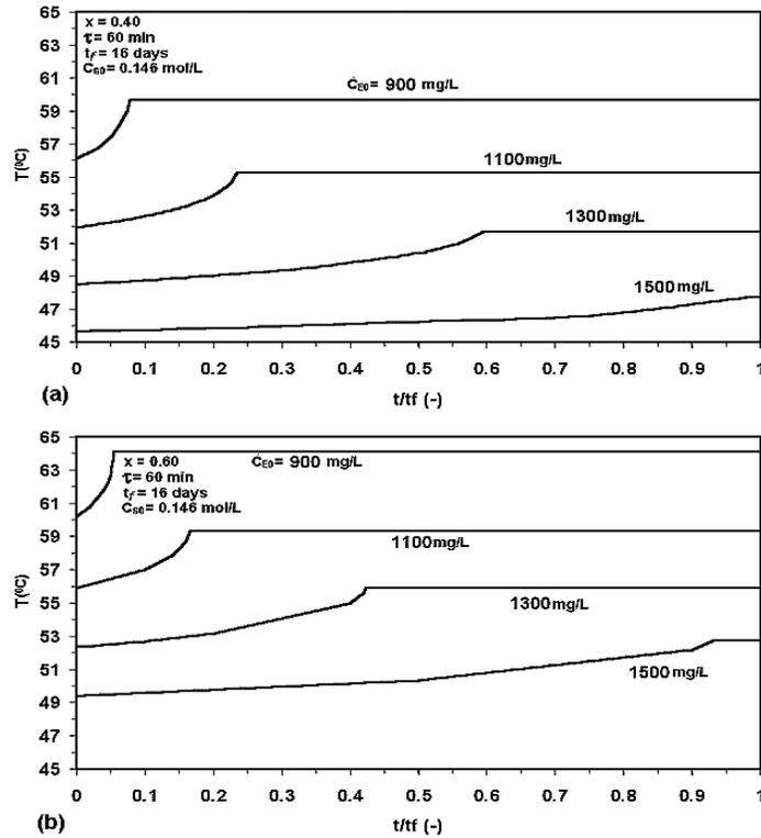
Fig. 7: Temperature profiles of an immobilized mesophilic lactose hydrolysis (a) CSTR, (b) PFR at different enzyme concentration and operating period of 16 days at a residence time of 60 min.
