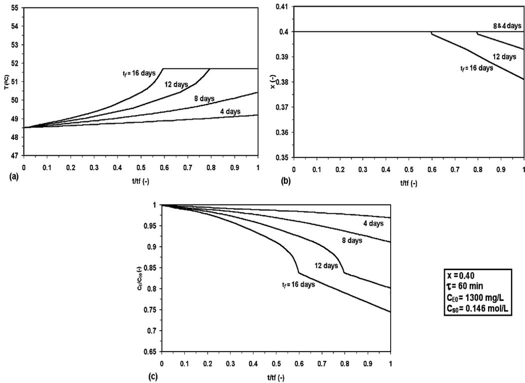
Fig. 1: (a) Temperature profiles, (b) Conversion profiles, (c) Activity profiles of an immobilized mesophilic lactose hydrolysis CSTR at different operating periods, residence time of 60 min and enzyme concentration of 1300 mg/L.
