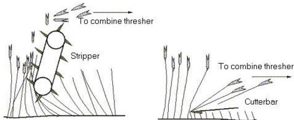
Fig 1. New and traditional technology of grain harvesting.
