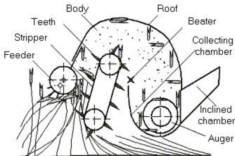
Fig. 3. The structural drawing of the stripper header.
