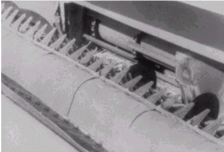
Fig. 8. View of the toothed edge of the collecting chamber.
