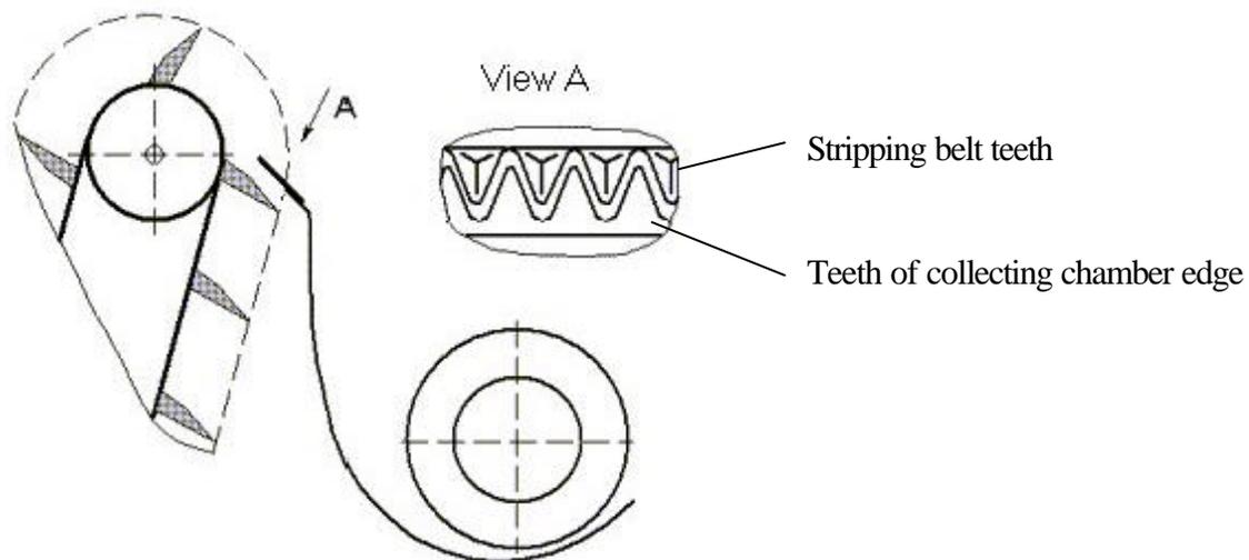
Fig. 6. Proposals for changing the upper edge of the collecting chamber wall.
