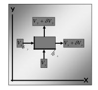
For a soil with permeability k<sub>x</sub> and k<sub>y</sub> in the x and y directions respectively, Laplace's equation for two-dimensional seepage becomes
