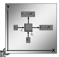
Two-dimensional steady flow of the incompressible pore fluid is governed by Laplace's equation which indicates simply that any imbalance in flows into and out of an element in the x direction must be compensated by a corresponding opposite imbalance in the y direction.
