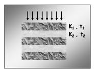
The flow rate q through area A of each layer is the same. Hence the head drop across a series of layers is
