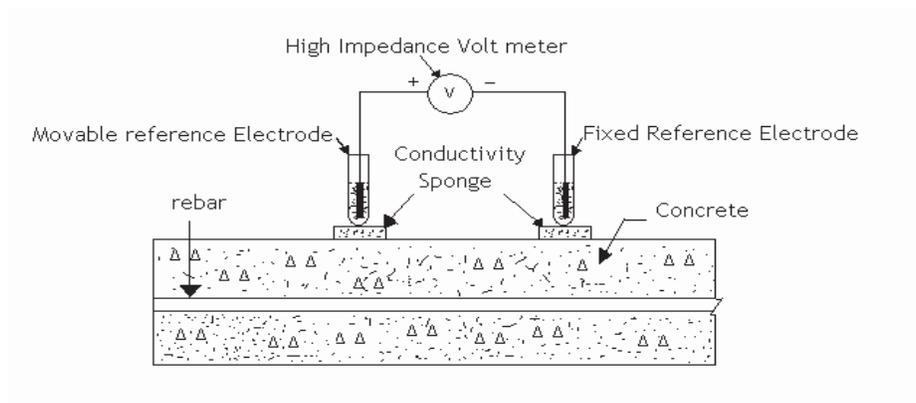
**Figure 2.** Schematic representation of surface potential (SP) measurements
