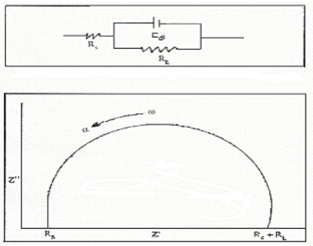
**Figure 9.** Nyquist Plot for steel in concrete
