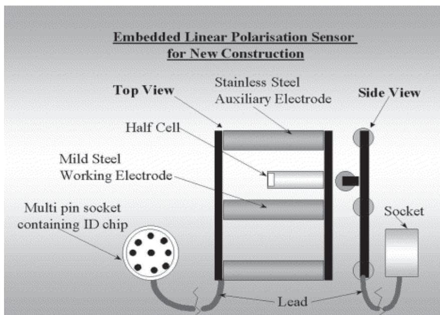
**Figure 6.** Embedded linear polarization sensor for new construction
