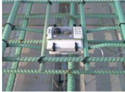
**Figure 10.** ECI sensor during operation
