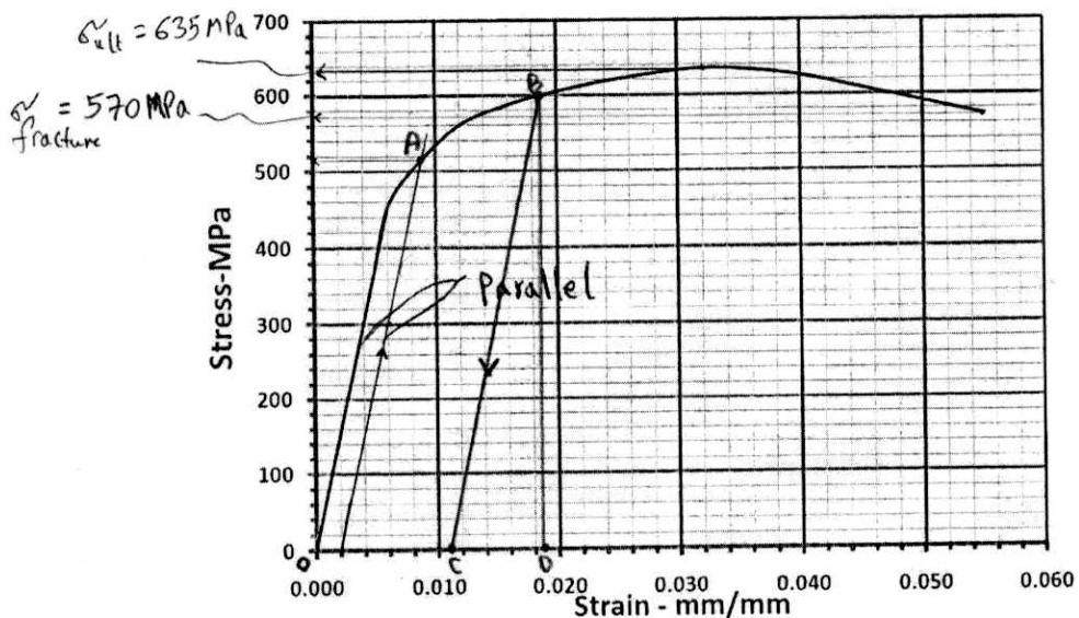
$$\text{The modulus of elasticity, } E = \frac{300 \text{ MPa} - 0}{0.004 \frac{\text{mm}}{\text{mm}} - 0} = 75 \times 10^9 \text{ Pa. } \quad (3)$$
