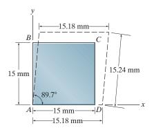
2-23. A square piece of material is deformed into the dashed parallelogram. Determine the average normal strain that occurs along the diagonals AC and BD.
