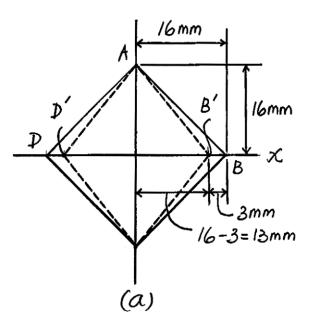
\*2-12. The piece of rubber is originally rectangular. Determine the average shear strain  $\gamma_{xy}$  at A if the corners B and D are subjected to the displacements that cause the rubber to distort as shown by the dashed lines.
