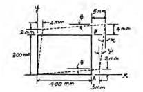
**2–19.** The piece of plastic is originally rectangular. Determine the shear strain  $\gamma_{xy}$  at corners D and C if the plastic distorts as shown by the dashed lines.
