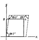
•2–25. The guy wire AB of a building frame is originally unstretched. Due to an earthquake, the two columns of the frame tilt  $\theta=2^{\circ}$ . Determine the approximate normal strain in the wire when the frame is in this position. Assume the columns are rigid and rotate about their lower supports.
