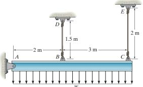
Since the vertical displacement of end C is small compared to the length of member AC, the vertical displacement  $\delta_B$  of point B, can be approximated by referring to the similar triangle shown in Fig. a
