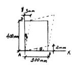
•2-13. The piece of rubber is originally rectangular and subjected to the deformation shown by the dashed lines. Determine the average normal strain along the diagonal DB and side AD.
