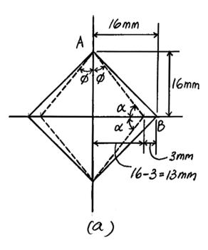
**2–11.** The corners B and D of the square plate are given the displacements indicated. Determine the average normal strains along side AB and diagonal DB.
