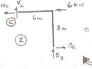
Writing three equations of equilibrium for the frame and supplementing this by a moment equation about a for half the frame.
