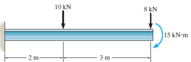
6-6. Draw the shear and moment diagrams for the overhang beam.
