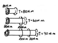
\*5-8. The solid 30-mm-diameter shaft is used to transmit the torques applied to the gears. Determine the absolute maximum shear stress on the shaft.
