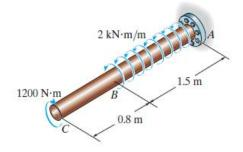
The internal torque for segment BC is constant  $T_{BC} = 1200 \text{ N} \cdot \text{m}$ , Fig. a. However, the internal torque for segment AB varies with x, Fig. b.
