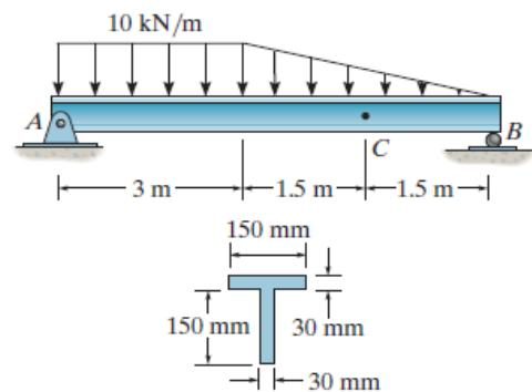
7-42. The T-beam is nailed together as shown. If the nails can each support a shear force of 4.5 KN, determine the maximum shear force  $V$  that the beam can support and the corresponding maximum nail spacing  $s$  to the nearest multiples of 5 mm. The allowable shear stress for the wood is  $\tau_{allow} = 3$  MPa.
