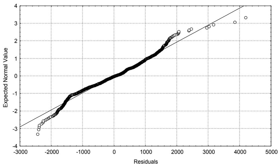
Figure 5: Normal probability plot for the prediction of the absolute maximum stresses for the pipe constructed on low density sand
