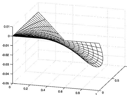
Figure 20. Clamped circular plate under uniform load: twisting moment.
