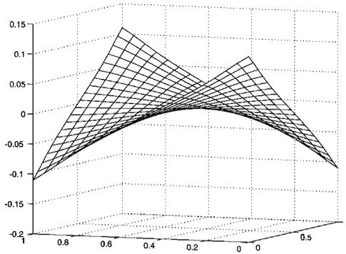
Figure 17. Uniformly loaded square plate supported only at the corners:  $M_{xy}$  distribution.
