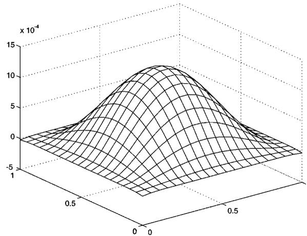
Figure 7. Uniformly loaded clamped square plate: deformed shape.
