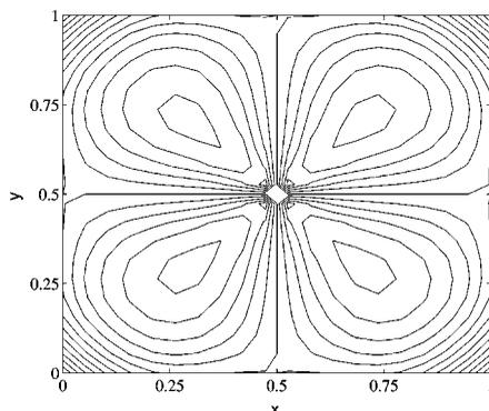
Figure 11. Concentrated load on a clamped square plate: twisting moment,  $m_{xy}$ , distribution.
