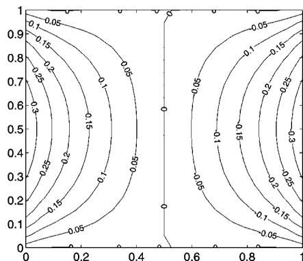
Figure 12. Uniformly loaded simply supported square plate: shearing force  $q_x$  distribution.
