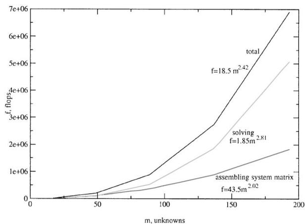
Figure 10. Floating point operations vs number of unknowns.
