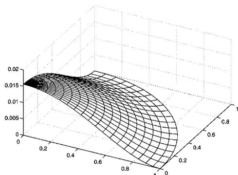
Figure 19. Clamped circular plate under uniform load: deformed shape.
