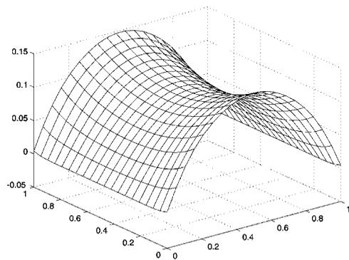
Figure 16. Uniformly loaded square plate supported only at the corners:  $M_x$  distribution.
