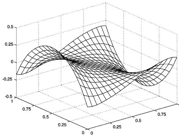
Figure 8. Uniformly loaded clamped square plate: shearing force  $q_x$  distribution.
