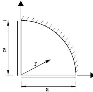
Figure 18. Quarter of a clamped circular plate.
