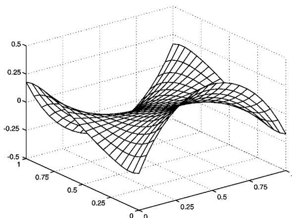
Figure 9. Uniformly loaded clamped square plate: shearing force  $q_y$  distribution.
