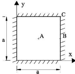
Figure 5. Clamped square plate.
