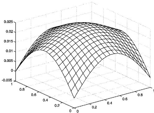
Figure 15. Uniformly loaded square plate supported only at the corners: deformed shape.
