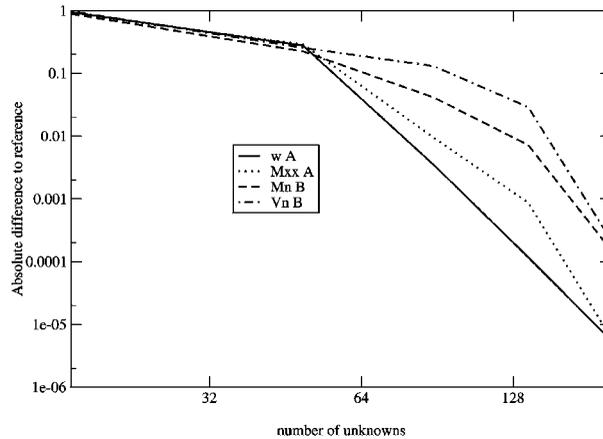
Figure 6. Convergence of the results for the uniformly loaded clamped square plate shown as the absolute differences to those of Reference [33].
