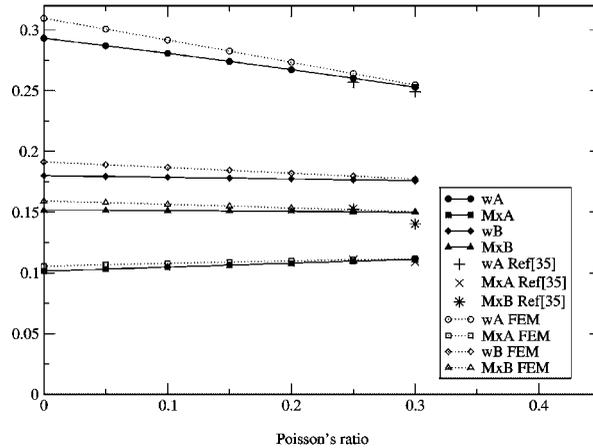
Figure 14. Uniformly loaded square plate supported only at the corners: effect of  $\nu$ .
