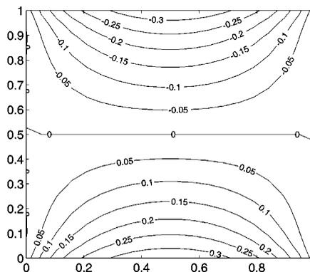
Figure 13. Uniformly loaded simply supported square plate: shearing force  $q_y$  distribution.
