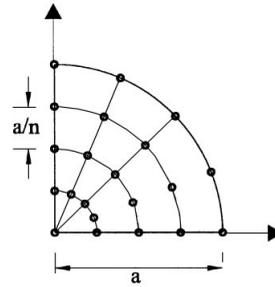
Figure 4. Distribution of collocation points used in the tests on circular plates.
