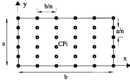
Figure 3. Distribution of collocation points used in the tests on square plates.
