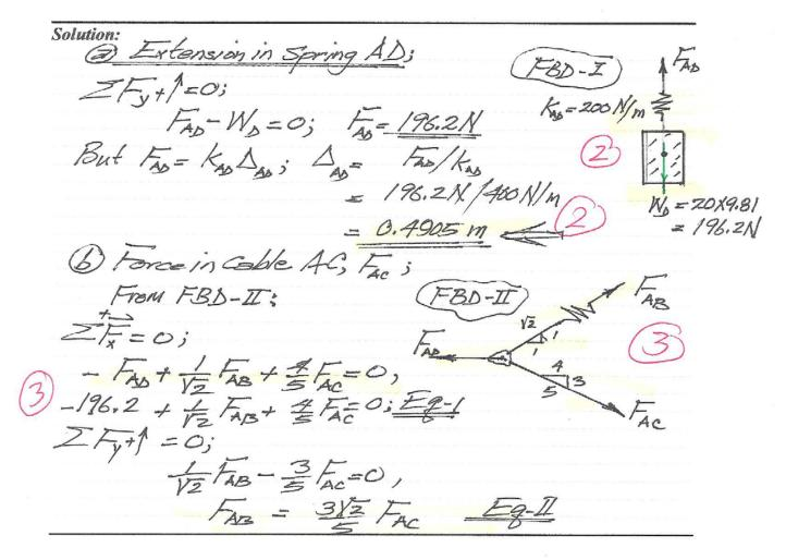
Solution: Substituting for Fas in Eg-I; -196,2 + 1/5 (3/2) Fac + 3 Fac = 0 FAC= 140.143/ 3 1 The distance between Aand B before Mp is added to the system; We have; FAB - 31/2 FAC - 31/2 (140.143) = 118.915 N 25 But FAR = KAB DAB : AB = FAB = 118.915N/200 N/m 3 and  $A_{AB} = L_{AB} - L_{AB}$ Where  $L_{AB} = \sqrt{4^2 + 4^2} = 5.657 \text{ m}$ and  $L_{AB}' = \text{distance between A and B}$ before  $M_{b}$  is added to the system. in LAR - LAR - DAR - 5.657 - 0.595 = 5.062 M
