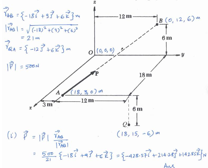
(ii)  $\vec{M}\vec{a} = \vec{7}\vec{a}\vec{A} \times \vec{\vec{l}} = \{-12\vec{\vec{l}} + 6\vec{k}\}x\{-428.57\vec{l} + 214.28\vec{j} + 142.85\vec{k}\}$   $= (-12)(-428.57)(-\vec{k}) + (-12)(142.85)(\vec{i})$   $+ (6)(-428.57)(\vec{j}) + (6)(214.28)(-\vec{l})$   $= \{-3000\vec{l} - 257\vec{l} - 5143\vec{k}\} N-m$   $|\vec{M}\vec{a}| = \sqrt{(-3000)^2 + (-2571)^2 + (-5143)^2} = 6485N4-m$ Aug
