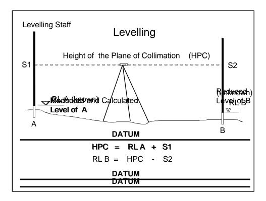
To determine elevation of selected point with respect to a point of known elevation: Elevation of A = 220.15 **BSA** +1.80= HI 221.95 = FS B - 2.45 = Elevation B 219.40 m = The elevation of any point lower than LOS, and the rod is visible from level, can be determined.
