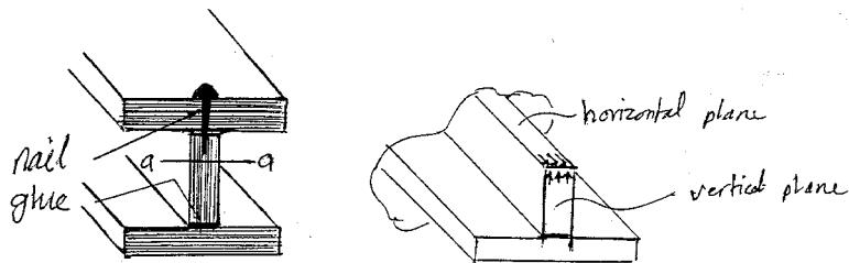
Note that for pure moment ( $M = \text{constant}$ ),  $V=0$  accordingly the shear stresses in vertical and horizontal planes are zero. and therefore no slipping and no need for nail or glue.
