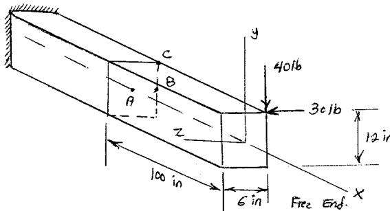
(a) Find the state of stress at points A, B, and C which are contained in a plane 100 in from the free end
