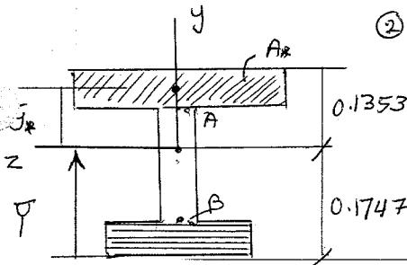
② calculate moment of inertia about  $z$ -axis (or N.A.)
