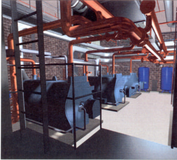
Fig. 15.2 3D CAD modelling helps in eliminating ambiguities that may creep around in 2D drawings (BSS, 1997)
