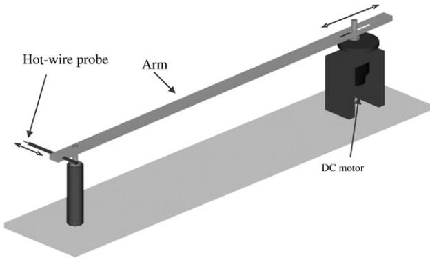
Fig. 1. 3D view of the calibration device.
