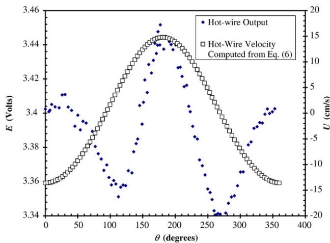
Fig. 4. Hot-wire output and velocity computed from Eq. (6).
